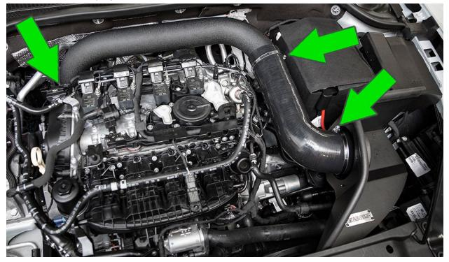
Using a T30 torx driver, completely tighten the intake pipe to the factory turbo heatshield.
