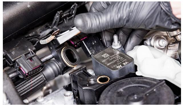
Using pliers or the factory hose clamp tool, release tension from the upper turbo inlet pipe coupler clamp and completely remove the turbo inlet pipe. Note: Pay close attention to the PCV breather return hose routing, you will need to re-install the new one in the same matter.
