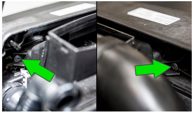
Separate the two halves of the air snorkel by releasing the two tabs on both sides and remove the front half from the vehicle.
