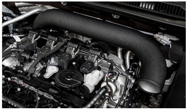
Reinstall coilpack, coilpack post, eyelets, coilpack harness connectors, and 10mm nuts.
