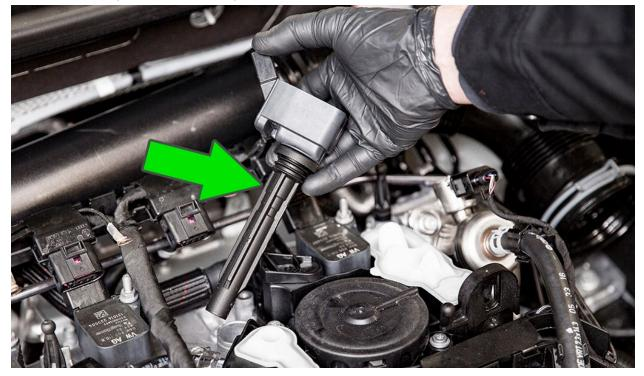
With the #3 cylinder coilpack out of the way, carefully push to release the o-ring sealed PCV breather return from the breather plate.
