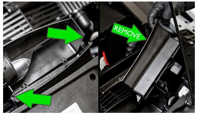
Locate and release the two tabs located on each side of the lower snorkel tube. Once loose,fully remove the air snorkel from the vehicle.
