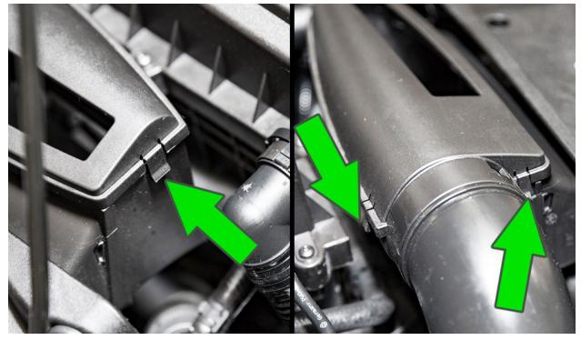
Locate and release the 3 tabs located on the air intake snorkel cover to remove it.
