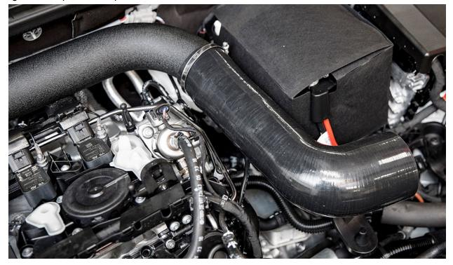
Connect the removed vacuum line to the 90 degree vacuum inlet located on the bottom of the 90 degree silicone hose.
