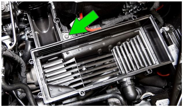
Carefully pull up on the lower airbox to release it from the grommet posts and remove it from the vehicle.
