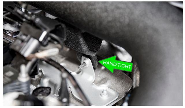
Route the new PCV breather return hose the same as factory as previously noted. Install back into the PCV breather plate and tighten the T30 torx bolt.
