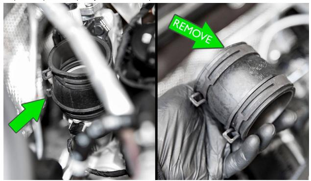
Install the new turbo inlet pipe coupler to the turbocharger with the included 50mm-70mm hose clamp. Tighten clamp.
