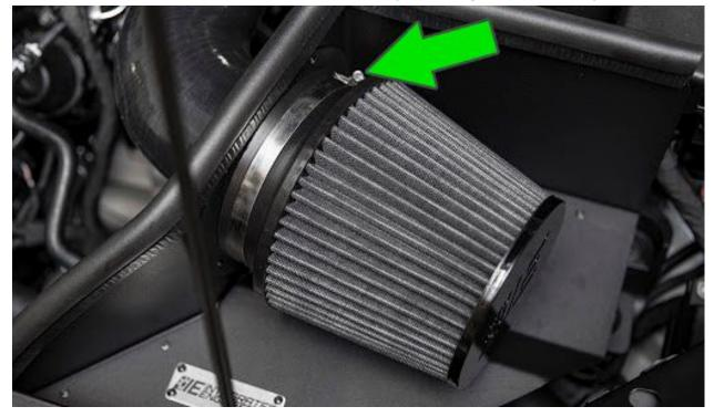
Verify all bolts, nuts, and harness clips are installed and tightened, all hose clamp connections are tight, and that your heat shield is fully installed. Start the car and inspect for any leaks or rubbing components. Reinstall the factory engine cover. Enjoy the performance, looks, and sound of your new IE Cold Air Intake!
