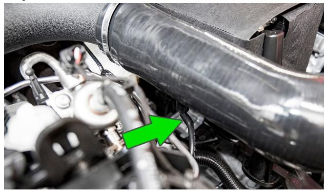
Line up the heatshield and install the rear of the velocity stack to the intake silicone with the supplied 80mm-100mm hose clamp. Do not tighten in this step.
