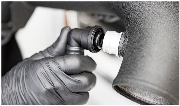
Install the new turbo inlet pipe into the turbo inlet silicone with the supplied 70mm-90mm clamp. Do not tighten clamp in this step.
