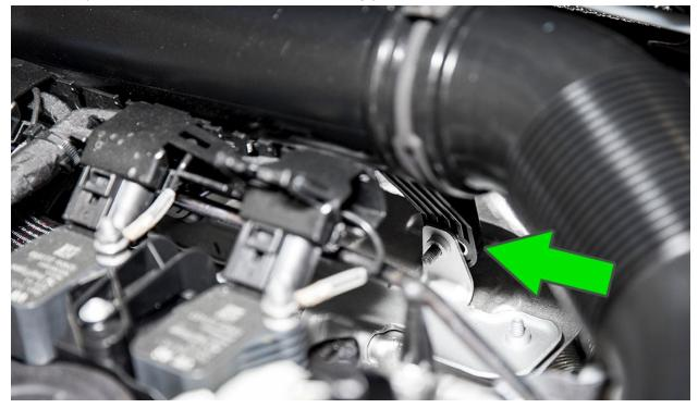
Using a 10mm socket, remove the 4 nuts located on the right hand side of the coilpacks.
