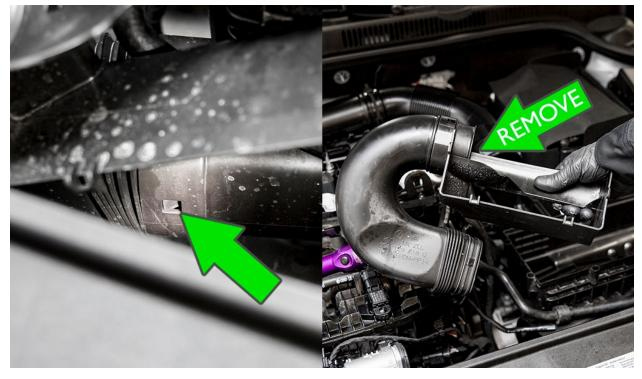
Using a T30 torx driver, remove the torx bolt from the lower airbox.
