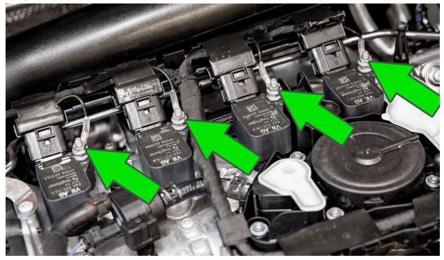
Carefully lift and remove all 4 eyelets from the coilpack posts.
