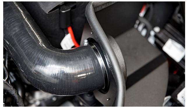
Line up the heatshield grommets with the grommet posts and push down to secure the heatshield.
