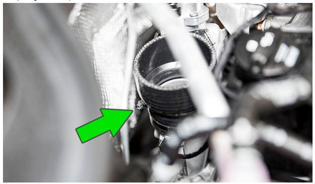
Push clip the new supplied PCV breather return hose to the new turbo inlet pipe.
