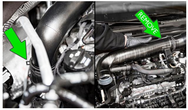
Using pliers or the factory hose clamp tool, release tension from the lower turbo inlet pipe coupler clamp and completely remove the coupler.
