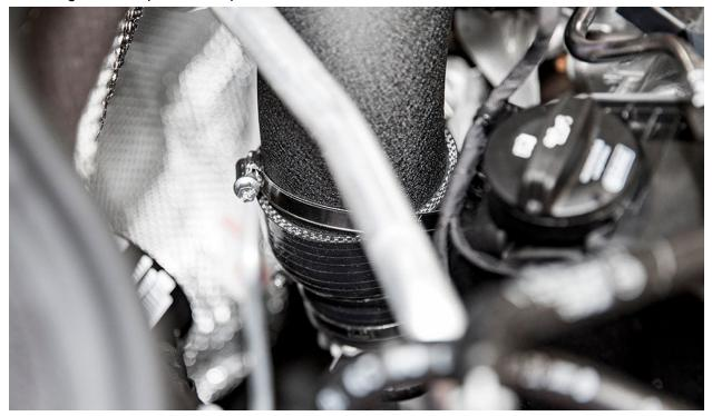
Reinstall the factory T30 torx bolt with the IE turbo inlet pipe, only tighten by hand in this step.
