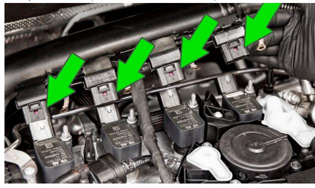
Carefully disconnect all coilpack harness connectors from the coilpacks.
