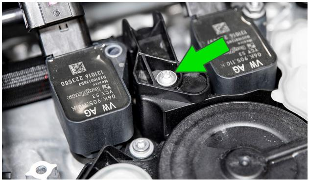
Pull to completely remove the #3 cylinder coilpack.
