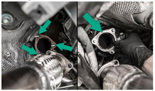
Install the IE downpipes to the CAT flanges with the included nuts, then tighten using 13mm sockets and crescent wrenches. Torque bolts and nuts to 19 ft-lb.
