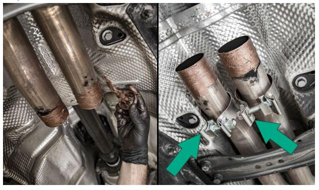
Line up the downpipe to CAT flange then install the slip-fit adapter to the factory catback. Repeat this step on both downpipes.
