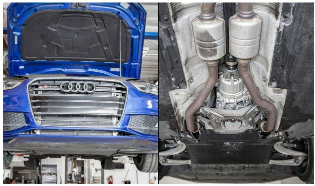
Begin the install by removing the transmission pan. Remove the 3 T25 bolts and loosen the 3 phillips head screws. Using a flathead screwdriver, remove the 2 plastic clips and remove the belly pan completely.
