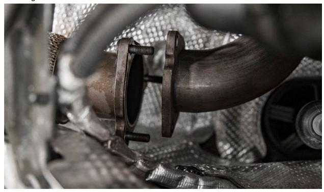
Using a 12mm socket, loosen the factory exhaust clamps and remove the downpipes from the vehicle.
