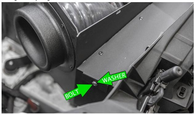
Install the remaining washer and M6 hex nut onto the isolator stud, tighten firmly using a 10mm socket.
