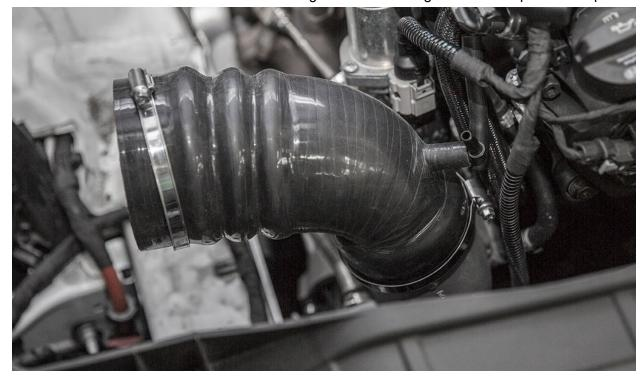
Re-install the vacuum line onto the barb on the new turbo inlet silicone.
