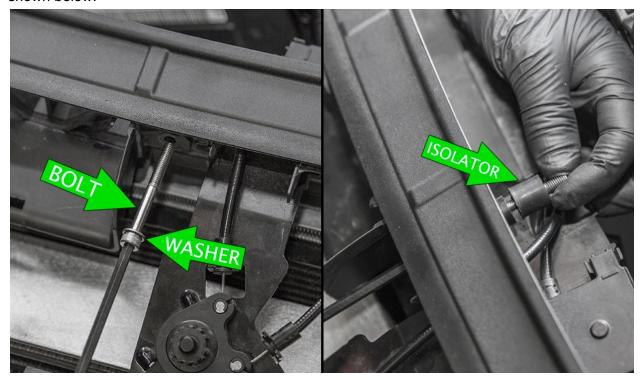
Position the intake channel into place and onto the isolator stud.
