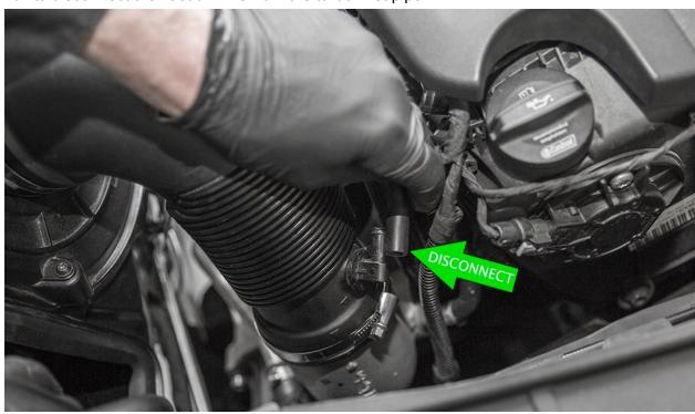
Disconnect the turbo inlet pipe from the airbox and turbocharger then remove it.
