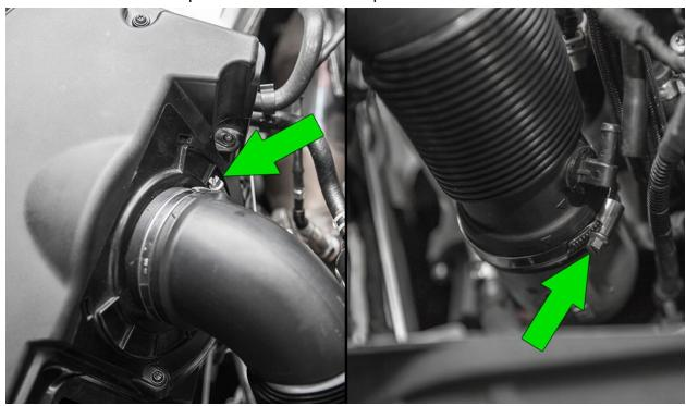
Pull to disconnect the vacuum line from the turbo inlet pipe.
