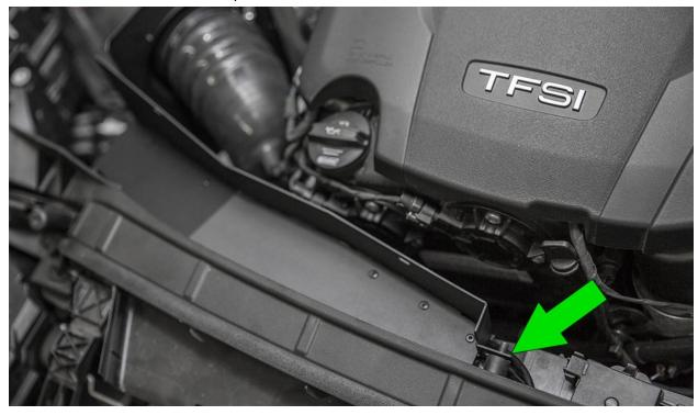
Install the channel to the heat shield assembly using an included washer and M6 button head bolt. Tighten firmly using a 4mm allen wrench.
