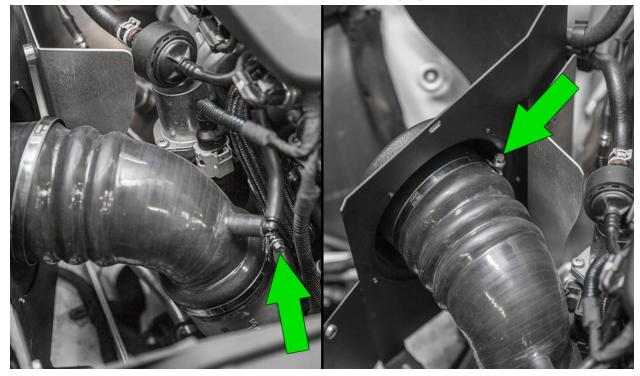
Slide the included M6x55mm allen bolt and washer through the open hole on the radiator support to the right of the intake inlet. Firmly tighten the included isolator stud to the bolt as
