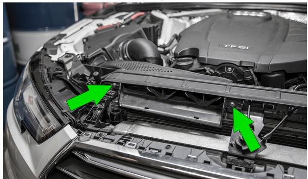
Lift from the corner to release and remove the intake snorkel completely.
