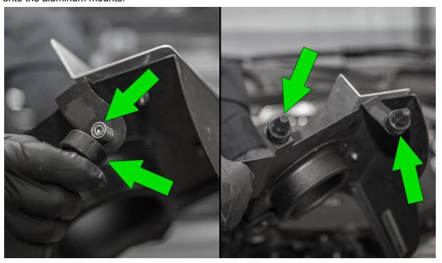
With the heat shield in place, (do not install the grommets to the vehicle in this step). Install the turbo inlet silicone to the velocity stack. Align the silicone so everything sits in place relaxed and without tension.
