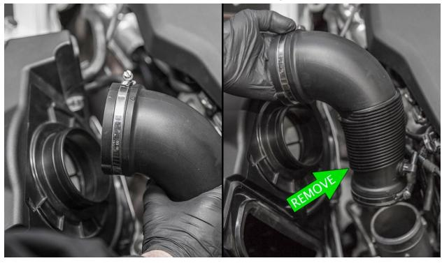
Carefully pull up to remove the factory airbox from the vehicle.
