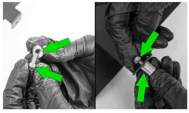
Using a 4mm allen wrench and 8mm socket, tighten both mount assemblies to the heat shield.
