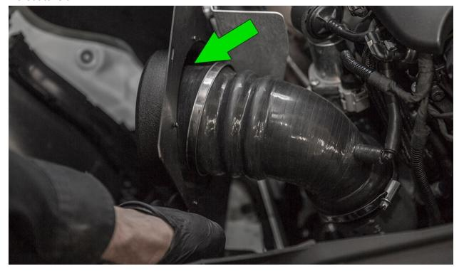
Align the grommets to the factory install points on the frame rail and firmly push down on the heat shield to lock them into place. This will install the same way as the stock airbox was previously.
