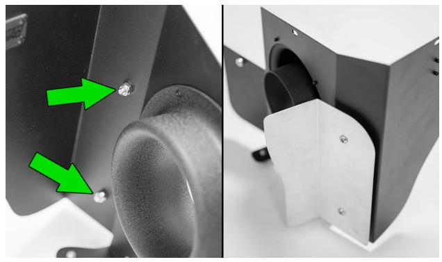
Reinstall the factory rubber grommets to the IE heat shield assembly by firmly pressing them onto the aluminum mounts.
