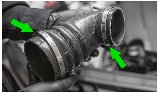
Seat the turbo inlet silicone over the turbocharger inlet. Do not tighten the clamp in this step.
