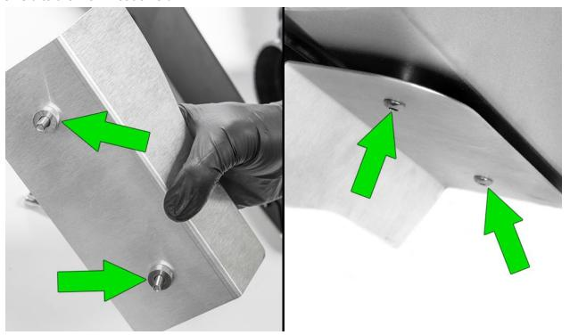
Install the included M6 locknuts and tighten the heat shield to the main heat shield firmly using a 10mm socket and 4mm allen wrench.
