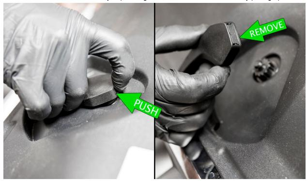
Slide forward and pull to remove the radiator support cowl.
