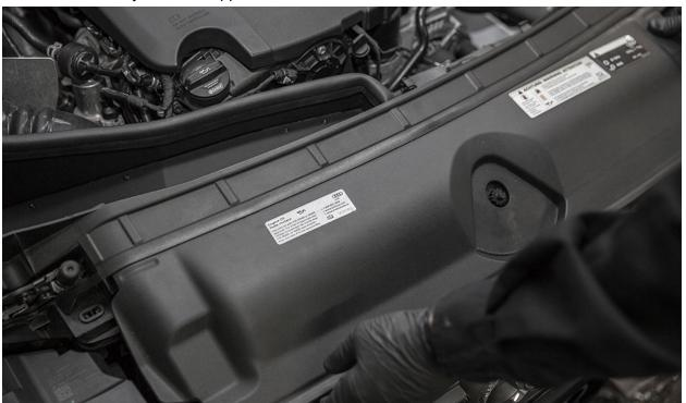
Verify all hose clamp connections are tight, and that your intake is fully installed. Start the car and inspect for any leaks or rubbing components. Enjoy the performance, looks, and sound of your new IE Cold Air Intake!
