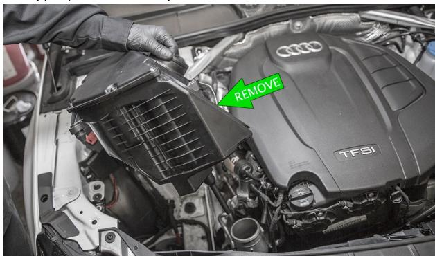
Carefully pull off the rubber grommets from the factory airbox, you will need to re-use these on your new IE intake. (Note: If you don't see the grommets on the intake box, they may have stuck and stayed in the frame rail, pull to remove them from the frame rail instead).
