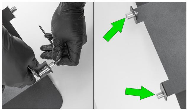
Use the included M6x18mm button head bolts and aluminum spacers to install the turbo heat shield to the main heat shield.
