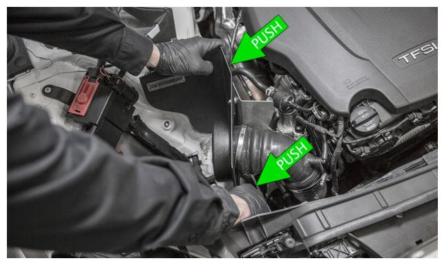
Double check the position of the intake silicone, make sure it is not pulling or bound and that it sits freely. Once you are happy with the intake position, firmly tighten both hose clamps.
