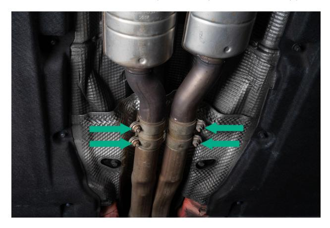
Remove four 13mm Midpipe Hanger bolts and hangers located on the inside of forward portion of the Midpipes on each side.
