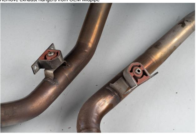
Reinstall exhaust hanger onto IE Midpipes
