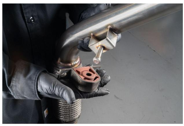
Raise front section of midpipe into engine bay and loosely fit exhaust hanger bolts and downpipe nuts.
