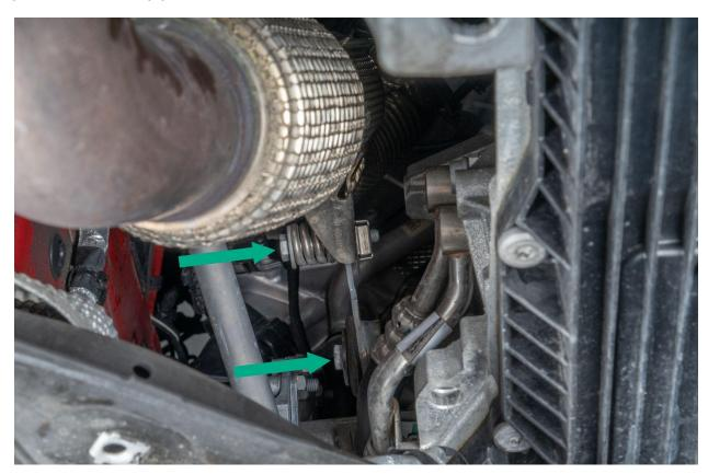
Remove two tripple square tens that fasten exhaust hanger to body on each side.
