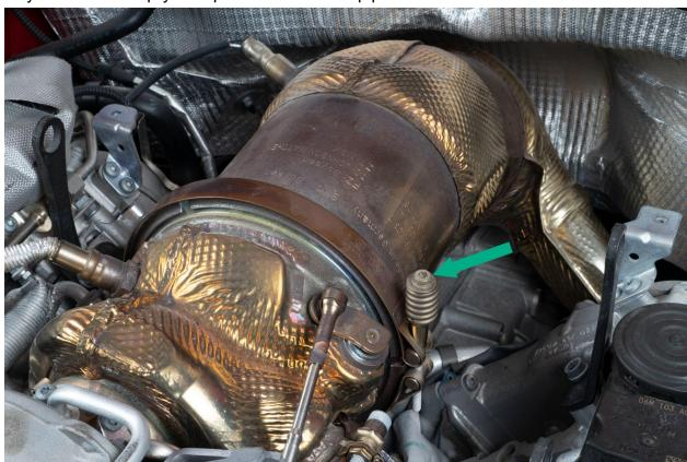
Remove six 12mm nuts that connect the downpipe to the midpipes. The two nuts in the back can be very difficult to gain access to, and remove. You will need to be creative with extensions, wobble sockets, and wrenches. Pushing the downpipe back towards firewall can also help with clearance.
