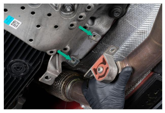
Remove OEM Midpipes by pulling out the bottom.
