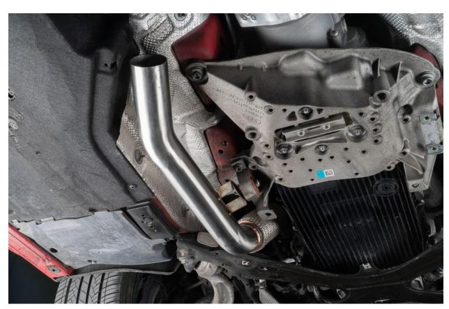
Slip exhaust clamps loosely over front portion of midpipes
