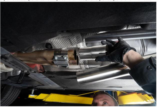
Slip IE Coupler onto IE Midpipes then position the reducer and two couplers into place.
