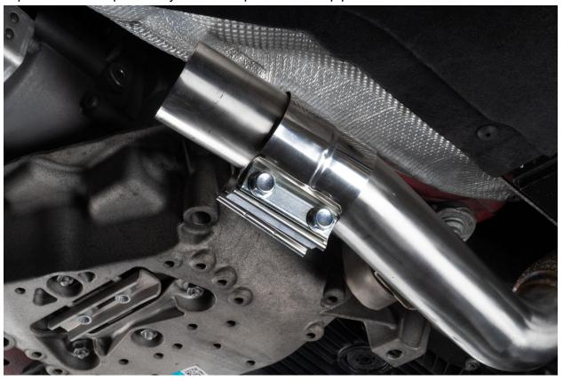
Remove OEM Exhaust clamp from rear portion of exhaust.
