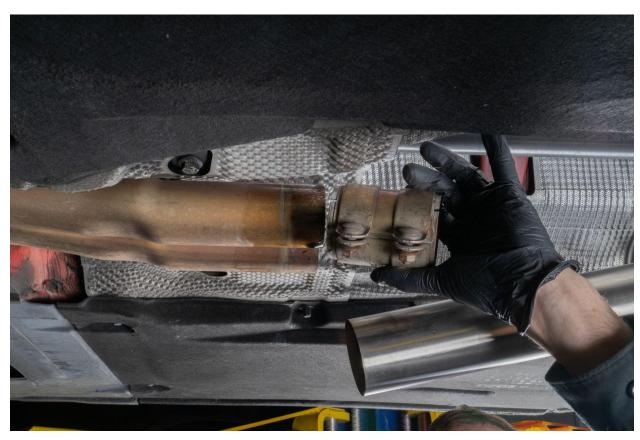
Slip exhaust clamp onto rear OEM portion of exhaust, then slip on coupler over OEM exhaust.
