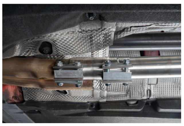
Ensure proper orientation of all parts, then tighten all Couplers, Exhaust Hanger Bolts, Downpipe V-Band and Downpipe bolts into place. Then reinstall underbelly pan and engine cover. Once all parts have been secured, enjoy the look and sound of your new IE Midpipes!
