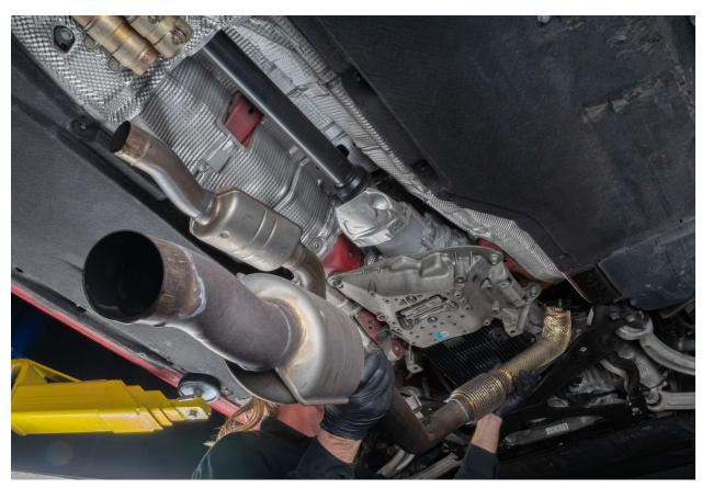
Remove exhaust hangers from OEM Midpipe
