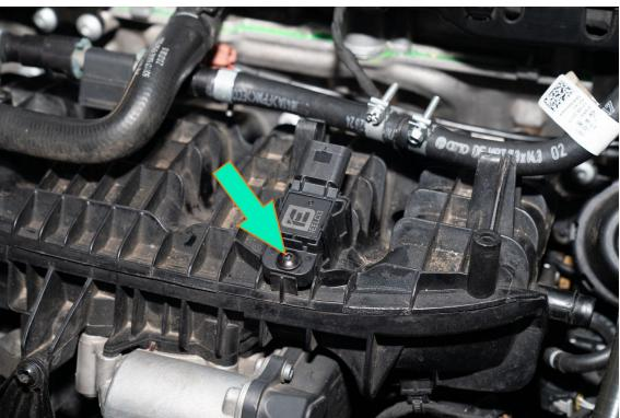
Reconnect the factory harness to the new sensor and lock it down by snapping the gray lock clip back into place. Make sure the connector is fully seated and locked before moving to the next step.
