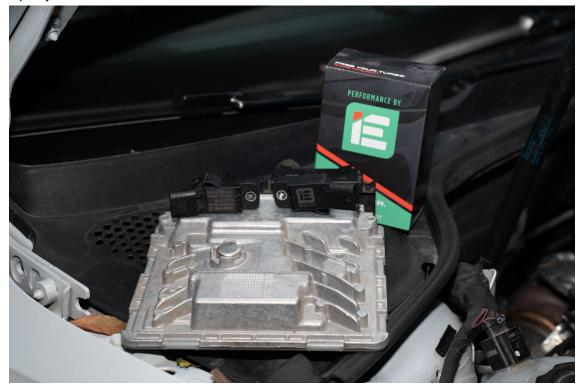
Align the new sensor into the factory position and press down to snap it into the mount retainers.
