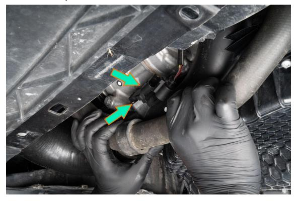
Reinstall the harness connector and verify its fully seated and locked onto the new IE PUT sensor.
