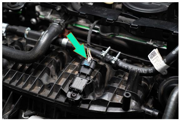
Pinch the sides of the connector locks and pull back to remove the connector harness from the sensor.
