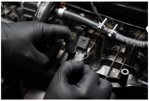
Apply upwards pressure to remove the sensor from the intake manifold. You may need to assist removal by gently prying the front corner of the sensor up with a flathead screwdriver.
