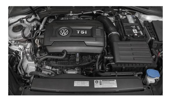
Begin by removing the engine cover to gain access to the intake manifold and disconnecting the MAP sensor harness. Unlock the harness connector by pulling up on the gray lock tab using a small flathead screwdriver or your thumbnail.
