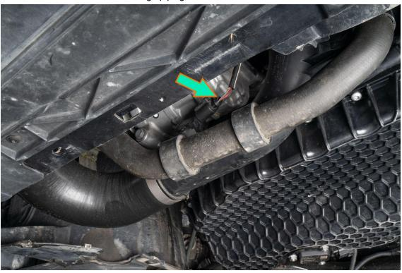
Use a T20 torx driver to remove both mount screws from the sensor.
