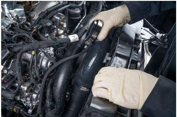
Install the spacer that was connected to the charge pipe behind intake manifold and charge pipe
