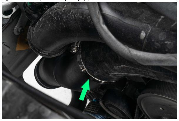
Loosely install hose clamps onto the silicone
