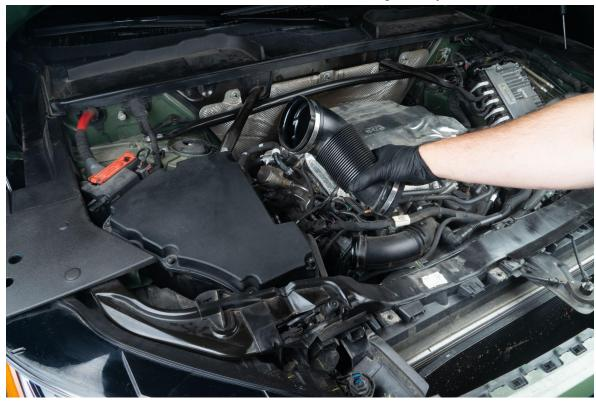
Remove Air Box from the vehicle by pulling straight up from three mounting tabs
