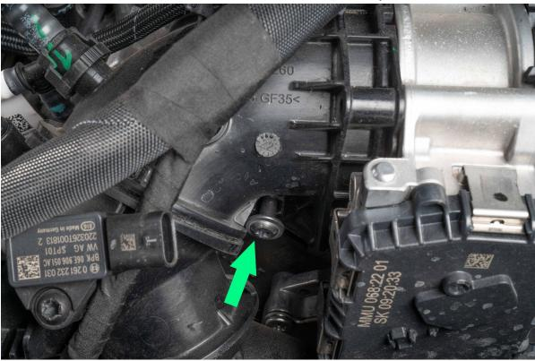
Remove two T30 screws underneath the turbocharger using a long T30 bit
