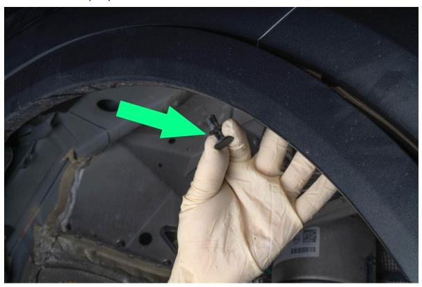
Remove one T25 screw from both sides connecting the front bumper and fender.
