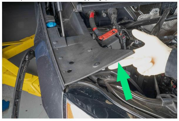
Remove two T30 screws that fasten the body to the radiator support from both sides.
