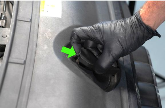
clips have been released, pull straight towards the front of the vehicle to remove.
