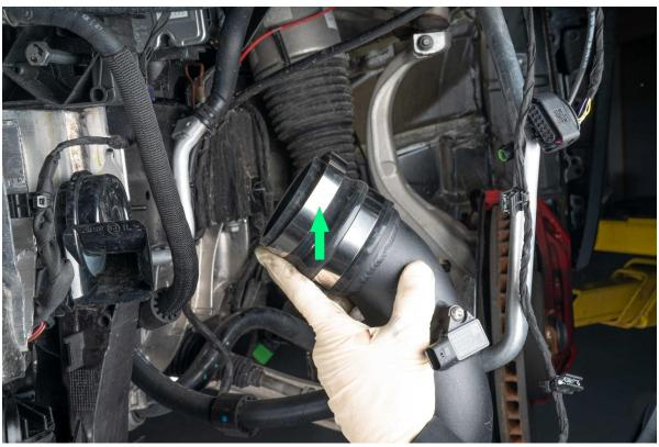
Install hose clamps to the silicone, slide silicone over the charge pipe
