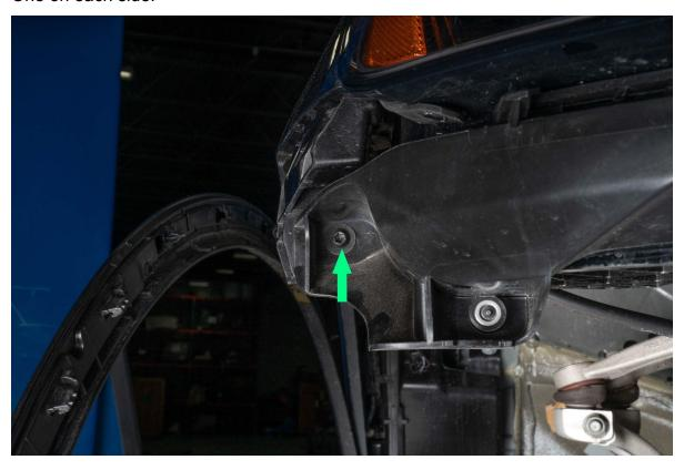
Remove plastic cover from both sides by pulling up from the corner.
