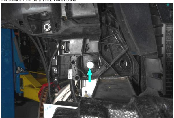
Remove MAP connector and hose connector to the charge pipe on the driver side by pressing in the gray tab then pulling the connector away from the plug
