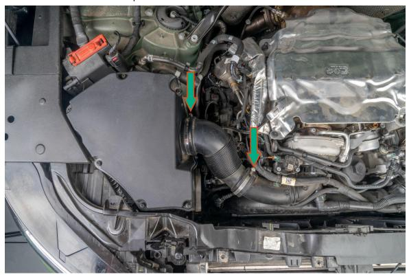
Remove the Intake Inlet Tube from Intake Box and engine bay
