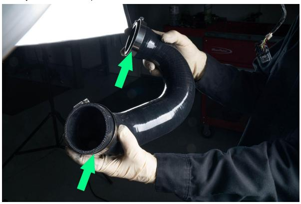
Install silicone tube to the intercooler end and tighten clamps securing silicone
