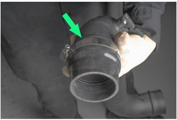
Attach 2nd hose clamp to charge pipe and place charge pipe into position by installing onto throttle body
