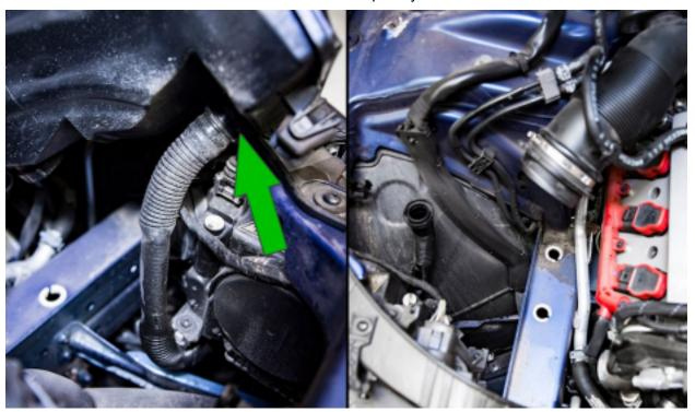
Remove two 10mm nuts from the HPFP housing.
