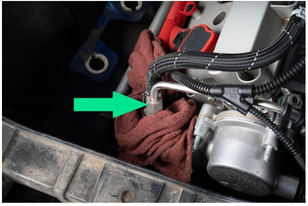
Using pliers, squeeze the clamp on the low pressure fuel line, move it up the line, then remove the line from the fuel pump.
