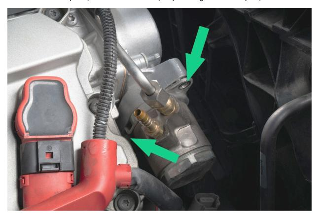
Remove both of the sensors from housing by pinching release tabs and pulling away.
