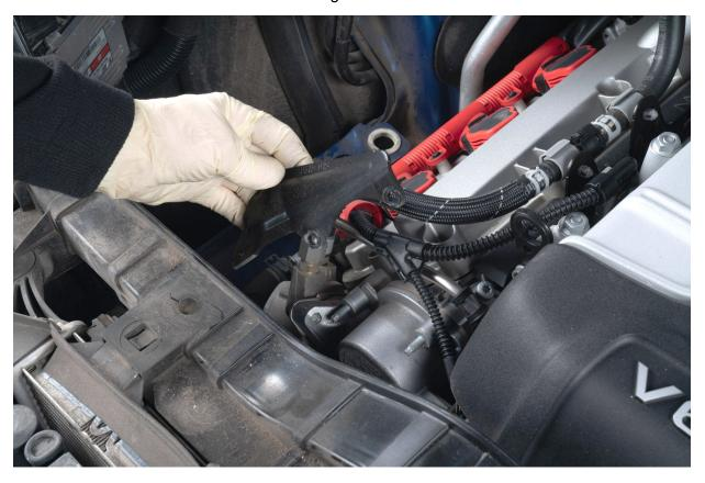
Remove the T30 screw from the top of the HPFP housing.
