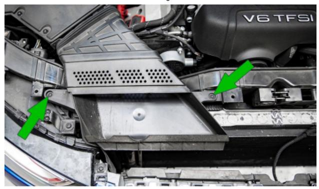
Disconnect the metal retaining clips and separate the inlet pipe from the airbox.
