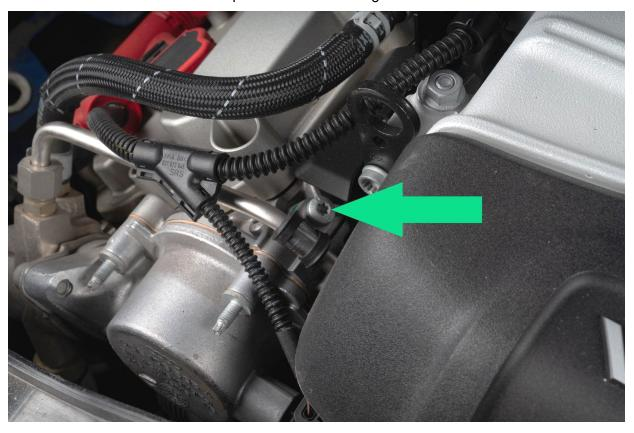
Place a rag around the line to catch any fuel, then slowly loosen the 17MM nut from the high pressure fuel line.
