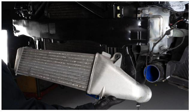
Remove two (One on each side) t30 screws that fasten the two lower intercooler mounts
