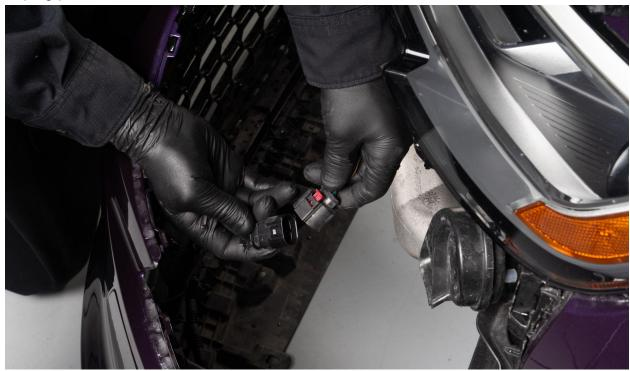
Clamp washer fluid hose above the connector, then disconnect headlight washer line.
