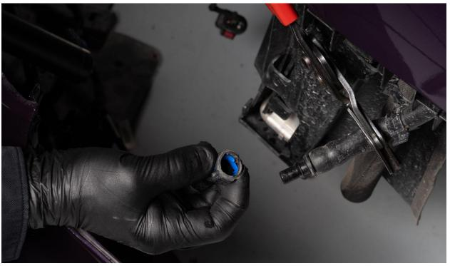
Set bumper aside, then remove two 7mm hose clamps on each side of the OEM Intercooler, then pull each hose off the intercooler
