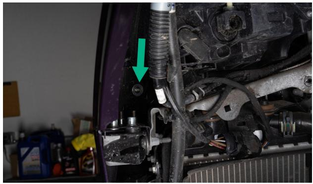
Remove the T25 torx screws under the front bumper on each side.
