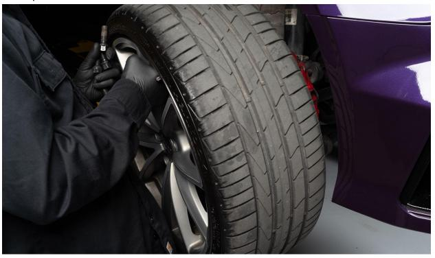
Remove 6 (Three on each side) T25 screws holding the fender liners to the bumper. If you prefer you can remove the fender liners entirely.
