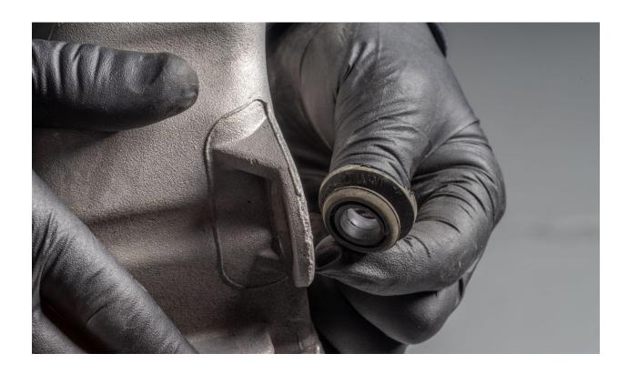
Using a Dremel and a sanding drum, carefully sand back about a 1/4 of an inch on each side in the marked locations of the core support.
