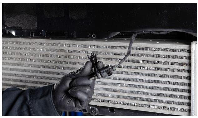
Unclip two wire retainer clips.
