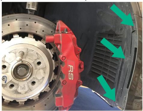
Pull back the front of the fender liner and remove the four (two on each side) T30 screws holding the bumper cover to the bottom of the front fender
