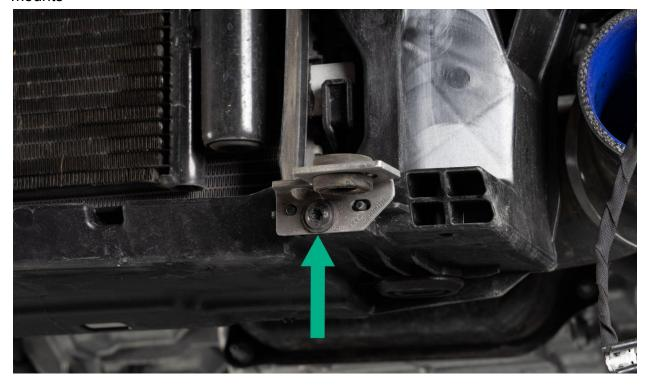
Remove factory grommets from top mounts of intercooler by removing center portion first, then pressing out surrounding grommet.
