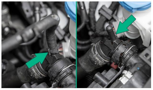
Install the new IE coolant hose & included clamps to the hardline line and then to the radiator hose barb. Install one side at a time as quickly as possible to limit the amount of coolant loss..
