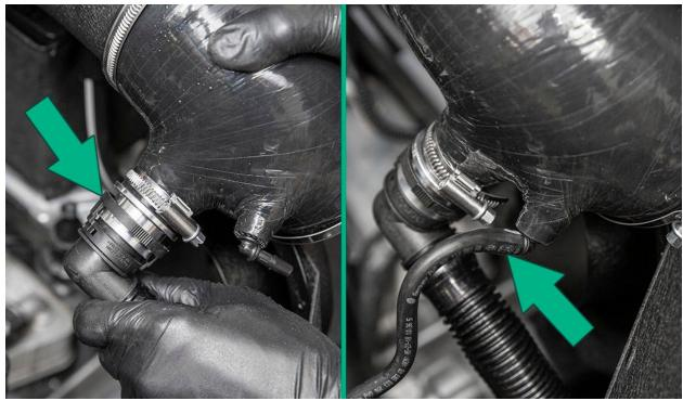
Fully seat the silicone couplers onto the turbo and IE heat shield. Align the silicone couplers and intake pipe so everything sits in place relaxed and without tension. Once you are happy with the intake position, firmly tighten all the hose clamps.
