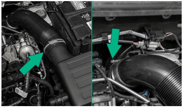
Completely remove the intake hose from the vehicle.
