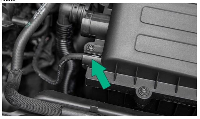
Carefully release the coolant line from the retaining clips by carefully pulling up on the hose.
