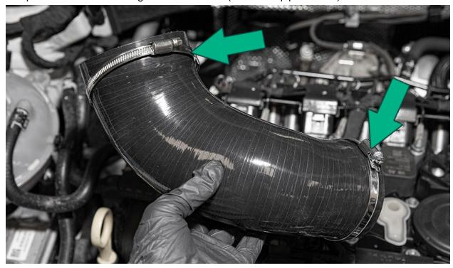
If installing on IE turbo inlet pipe, loosely install the included 80-100mm to the intake side and the 70-90mm hose clamp included in your IE turbo inlet pipe kit to the turbo side of the long IE turbo inlet silicone (IE Turbo Inlet version).
