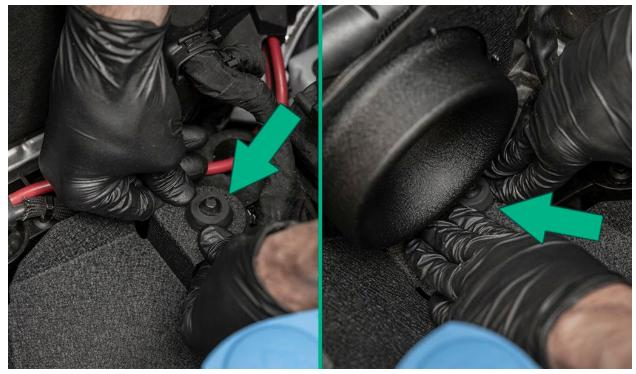
Secure the IE heat shield to the passenger side radiator support with the included button head bolt and washer. Tighten with a 4mm allen wrench.
