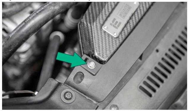
Install the included button head bolt and washer into the CF threaded insert on the driver side with a 4mm allen wrench.
