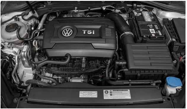
Start the installation procedure by carefully pulling up at the corners to remove your engine cover.
