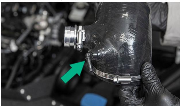
Your intake kit includes two long side intake silicones: one for the stock turbo inlet pipe and one for the IE Turbo Inlet Pipe (*sold separately*). The cast IE inlet pipe has a larger turbo side opening for the larger IE inlet. Identify the correct silicone for your setup in this step.
