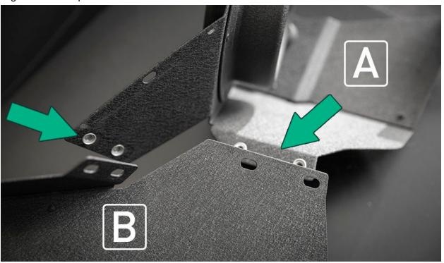
Thread X4 included button head bolts and washers through section B into threads of Section A. Tighten firmly with a 4mm allen wrench.
