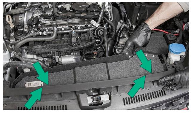
Line up the IE rubber mount grommets with the factory grommet posts and push down to lock them into place (X2).
