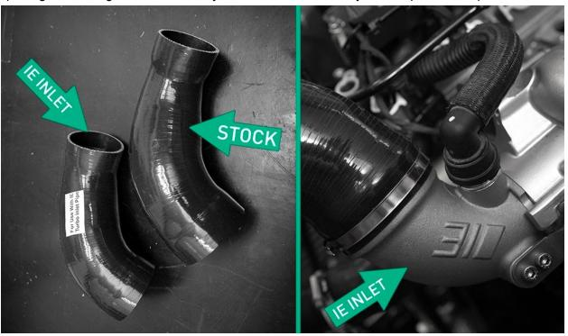
If installing stock turbo inlet pipe silicone, keep your IE inlet pipe silicone for the future upgrade.
