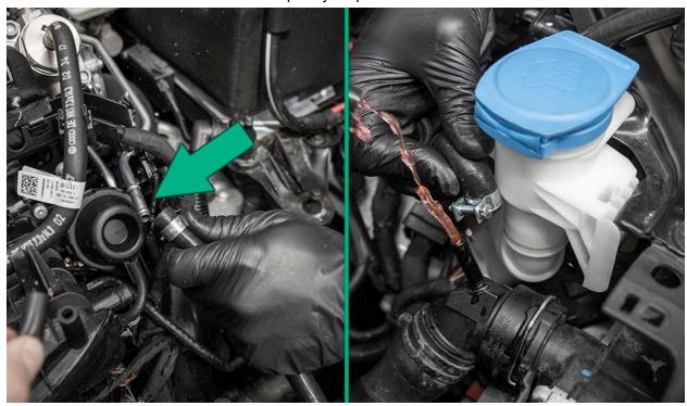
Once installed, firmly tighten both coolant line hose clamps.
