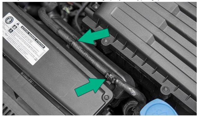
Using a T25 torx, remove both screws from the sides of the front air box inlet.
