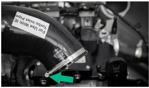
Assemble the long side of the IE intake pipe into the turbo side silicone hose. Orientate the silicone with the turbo and heat shield. *Do not tighten the hose clamps in this step.*
