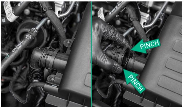
Carefully pull to remove the vacuum line from the airbox. *Do not stretch or tear this line, it will be reused.*
