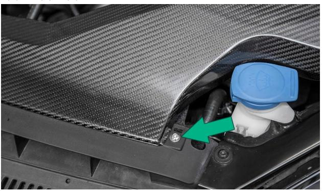
Reinstall the engine cover by aligning the grommets and pressing down to lock them in.
