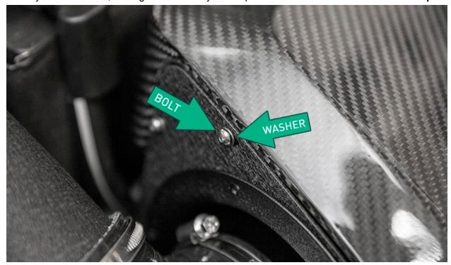
Retighten the button head bolt on the passenger side with a 4mm allen wrench.
