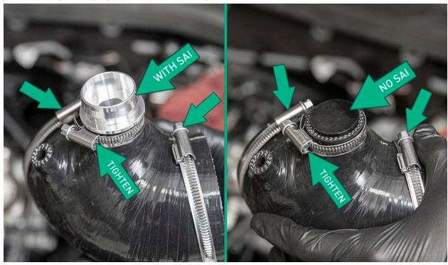
Install the included vacuum fitting into the short IE intake silicone.
