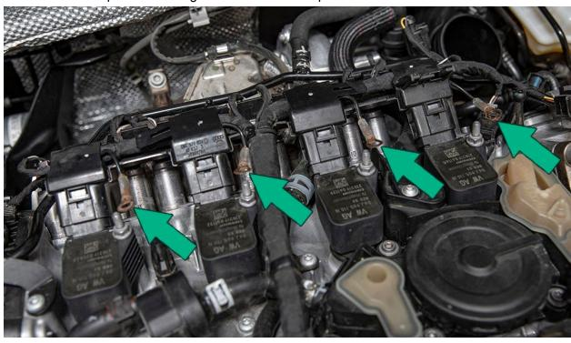
Carefully disconnect the harness from all 4 coil packs.
