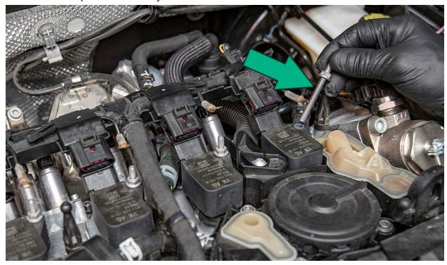
Pull up to remove cylinder one coil pack.
