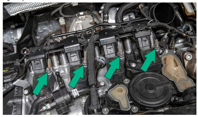
Remove all 4 coil pack harness grounds from the coil pack studs.
