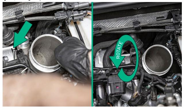
Tighten the factory mount bolt to the stainless mount arm with a T30 torx driver.
