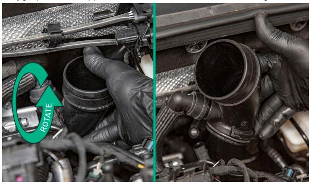
Pull and rotate back and forth to remove the breather hose from the turbo inlet pipe. *Note: This does not have a clip, just a tight o ring seal.*
