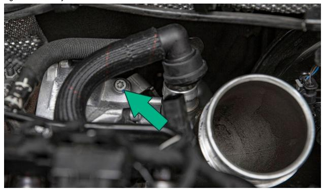
Press the breather hose onto the machined barb of your turbo inlet pipe.
