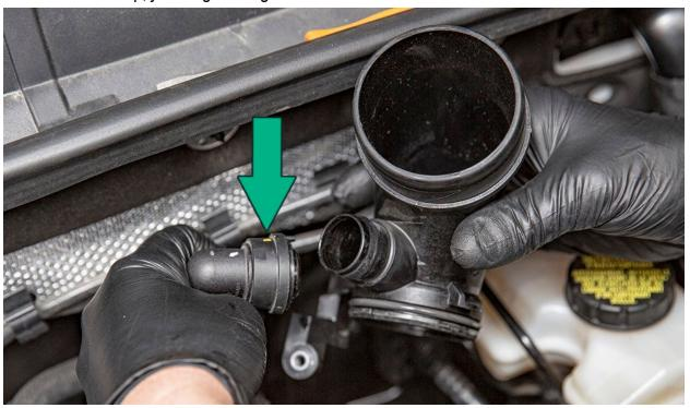
Install the included o ring onto the machined groove in your IE turbo inlet pipe.
