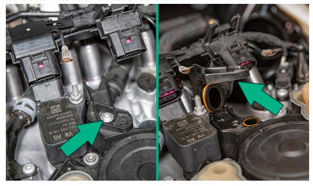
Loosen the mount bolt securing the factory turbo inlet pipe to the turbocharger with a T30 torx driver. *Note:* You do not need to fully remove this bolt, just loosen it until it's removed from the threads.
