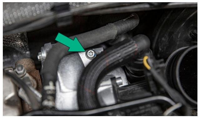
Firmly grasp the turbo inlet pipe and rotate clockwise to release from the turbocharger.
