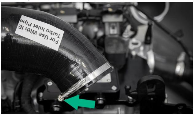
Install the clamp and intake silicone to the turbo inlet. Follow your cold air intake install guide to finish installation of your intake kit.
