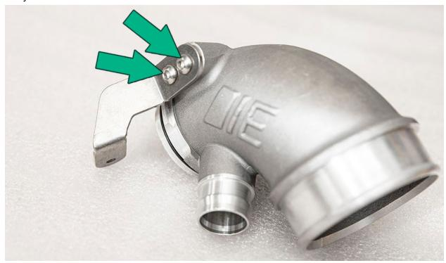
Align your new turbo inlet pipe collar with the channels in the turbocharger and fully seat the inlet into the compressor. Rotate the turbo inlet clockwise to lock into place. Note: This is a very tight fit, rotating into place takes some effort.
