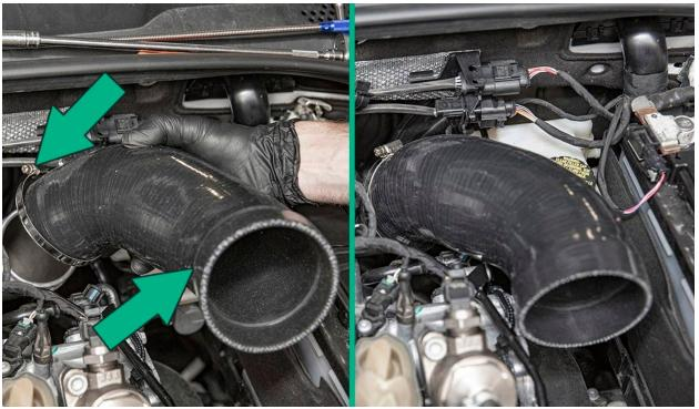
With the intake fully installed. Reinstall the engine cover by aligning the grommets and pressing down to lock them in.
