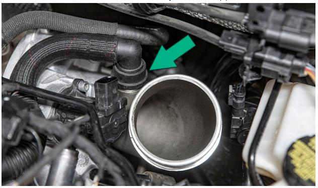
Completely reinstall your breather hose, coil pack, and coil pack harness in the reverse order of uninstall.
