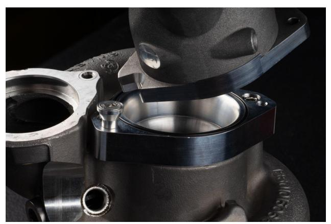
Use the button head screw to attach the inlet to the adapter. **IE Suggests adding Blue LocTite** to this thread during installation.
