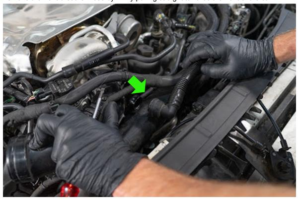
Remove two T30 screws holding on the factory turbo inlet to the turbo
