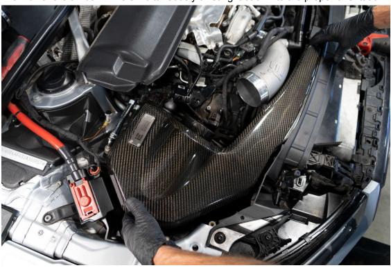
With the turbo inlet and the intake in place, rein at stall the radiator Allen bolts, silicone elbow, hose clamps, radiator cover, hood latch, and engine cover. Enjoy your new IE Turbo Inlet Pipe!
