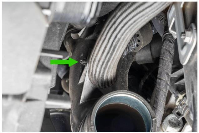
Remove the wiring loom clip located about halfway up the outlet pipe with a trim removal tool or flathead screwdriver.
