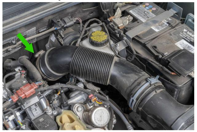
Gently lift up to remove the coolant hose from the mount clips on the intake inlet.
