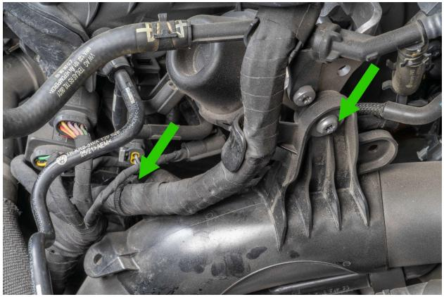
Depress both sides of the radiator fan shroud mount clips and pull fan shroud straight up to disconnect it from the radiator mount.
