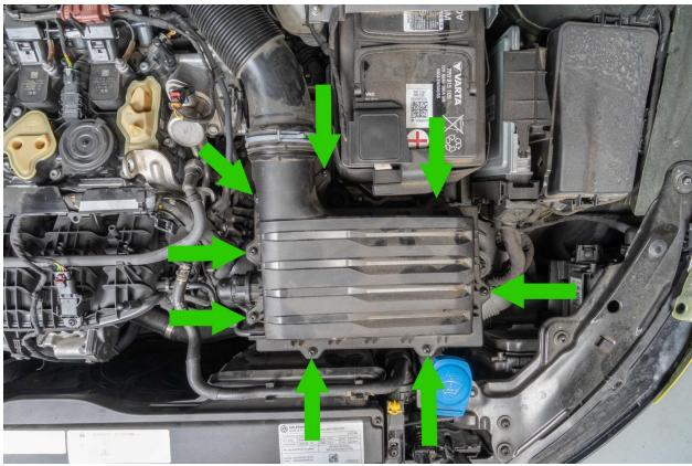
Remove all 8 mount screws from the airbox with a T25 torx driver.
