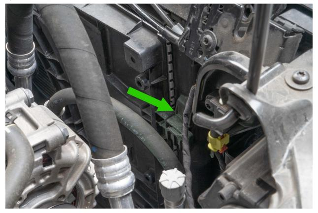
Remove radiator fan from engine bay
