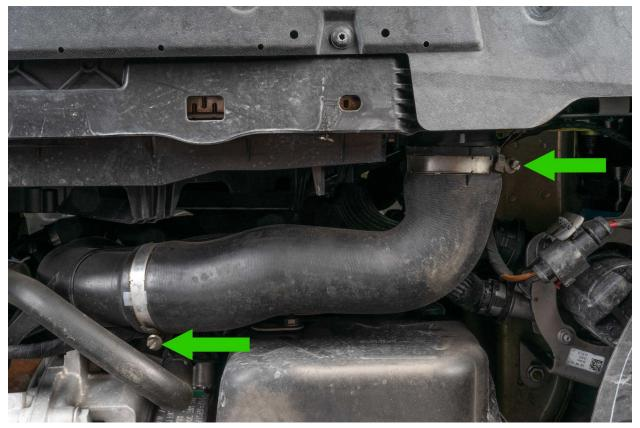
Remove the wire loom clip located by the turbo outlet pipe by pressing in on the center hole located on the back of the clip.
