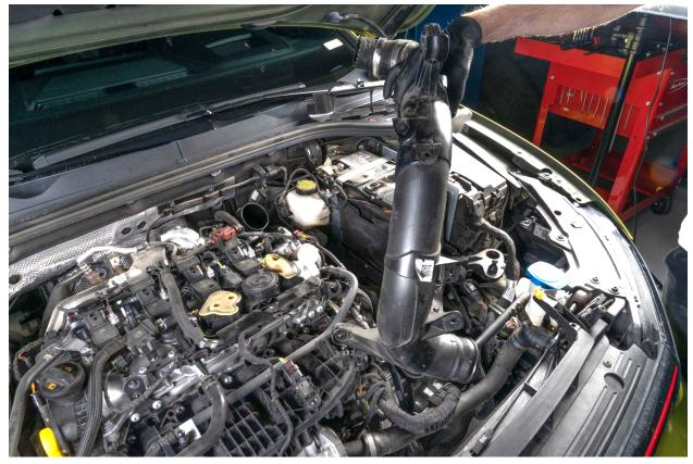
Remove both rubber grommets and bolts from the OEM Turbo Outlet Pipe and transfer them to your new IE Turbo Outlet Pipe.
