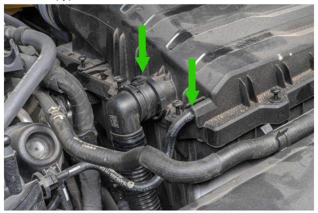
Loosen the rear intake hose clamp with a flathead screwdriver, then remove the intake box lid and intake hose together.
