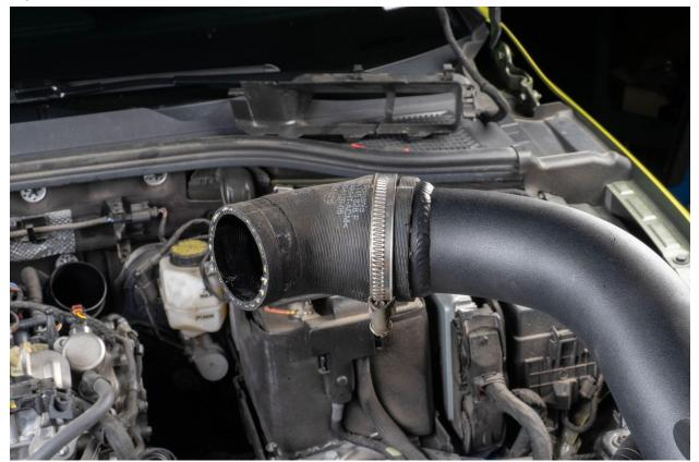
Drop IE charge pipe into place and orient silicone couplers, then make sure it aligns with all the proper fittings.
