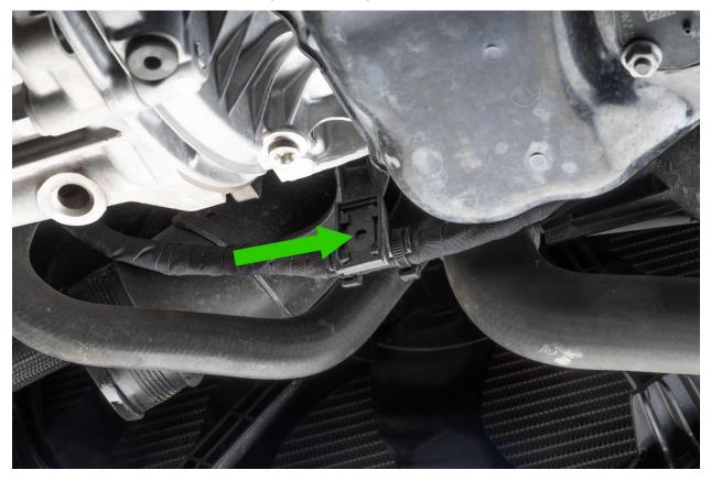
Remove the secondary air hose clip from the outlet pipe with a trim removal tool.
