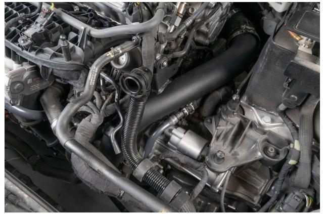
Verify your hose clamp connections, bolts and screws are tight. Double check mount clips are secured, electrical connectors are fully seated, and the radiator fan shroud is clear. Start the car and inspect for any leaks or rubbing components. Enjoy the performance and sound of your new IE Turbo Outlet Pipe!
