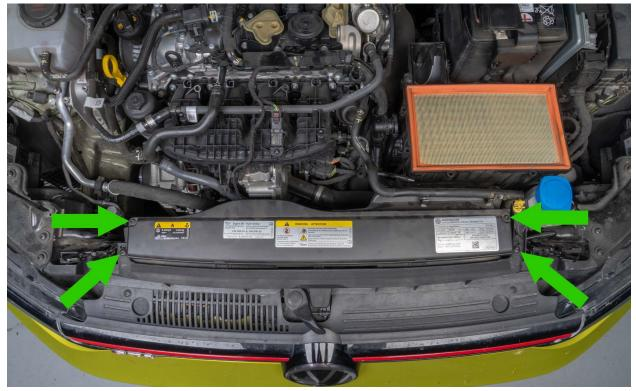
Push down on both mount tabs to release the air filter inlet from the radiator support.
