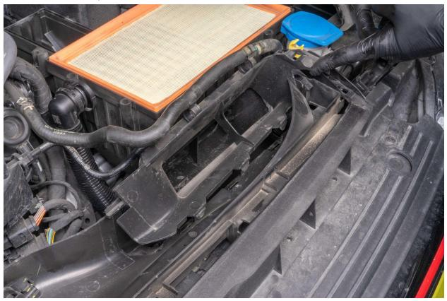
Remove the remaining air box by pulling straight to pop it off the 3 mount tabs.
