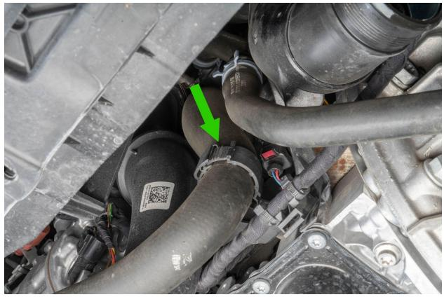
Remove the lower turbo outlet pipe mount bolt with a T30 torx driver.
