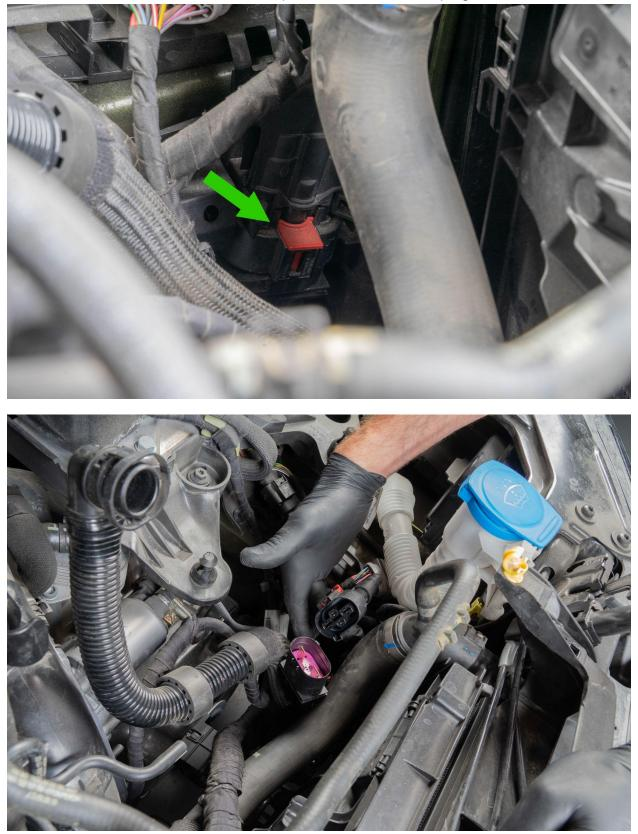
Disconnect the final wiring loom clip from the turbo outlet pipe with a flathead screwdriver. Remove the upper outlet pipe mount bolt with a T30 torx driver.
