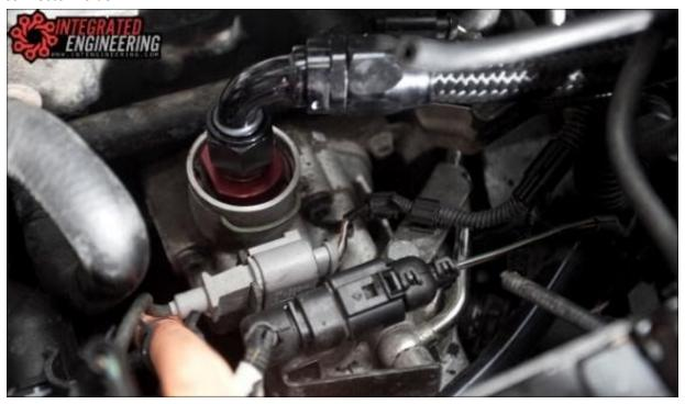
Place the supplied vacuum cap on the suction jet pump and use the supplied crimp clamp to secure the cap.
