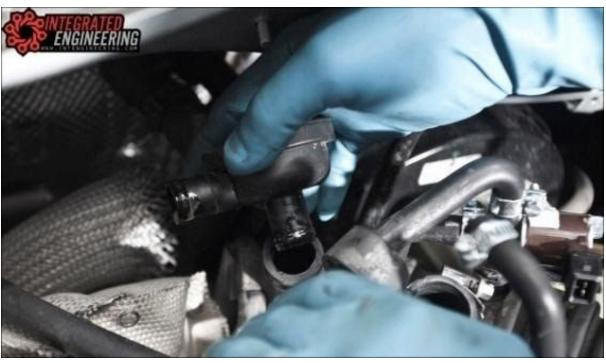
Install the supplied hose clamp and then the plug which eliminates the need for this valve. Tighten the clamp so that the plug is firmly secured in the turbo inlet boot.
