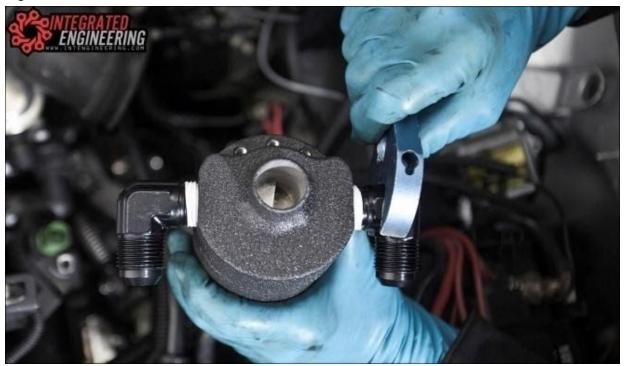
Install the catch can onto the bracket that is mounted to the firewall using the three supplied bolts with a 4mm allen wrench.
