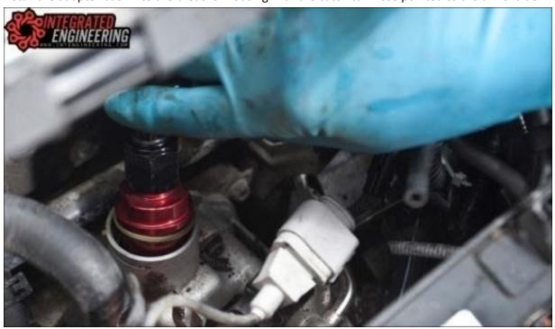
Re-Install the green U clip around the breather adapter and place the crank position sensor back into the connector holder.
