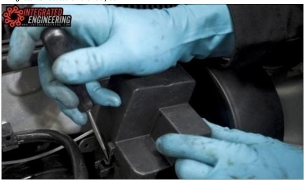
Remove the top cover of the relay box by pressing on the tabs located on both sides of the top half of the box. Remove the whole relay box by pulling forward on the tap located on the firewall and lifting up on the box.
