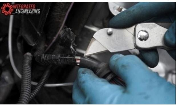
After the tape has been removed, carefully cut the grommet off of the harness and remove.
