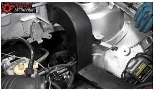
Remove the diverter valve from the inlet boot to gain access to the pressure regulating valve. Cut both of the factory crimp clamps from the pressure regulating valve and remove the valve from the inlet boot.
