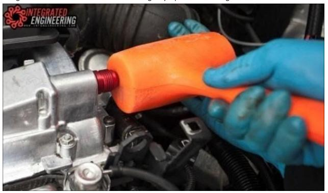
Install the last remaining line with the 45 degree fitting going to the valve cover, and tighten so that the fitting is in the downward position.
