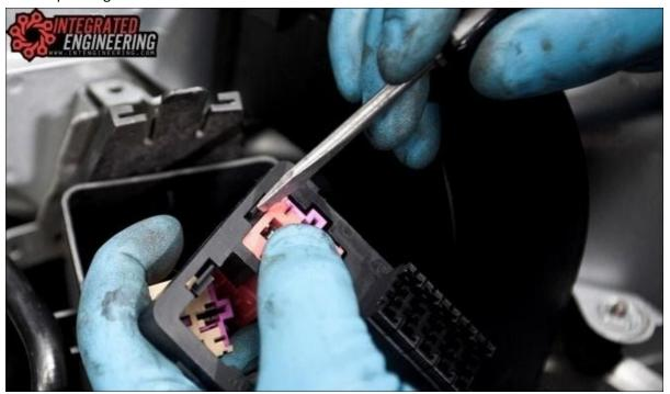
Pull the wiring harness and grommet out of the lower half of the relay box and discard the box. The box will no longer be used any more.
