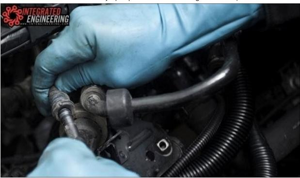
Locate the grey crank position sensor connector end, mounted on the oil breather housing and remove from the bracket by lifting up.
