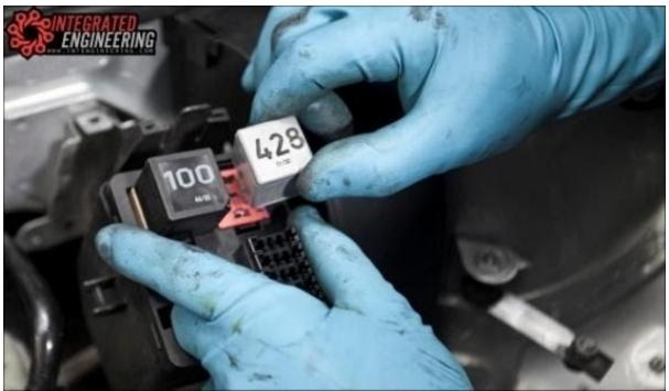
Release the connector ends that are housed in the top half of the relay box by pressing on the securing tab and pressing down on the connector end at the same time.
