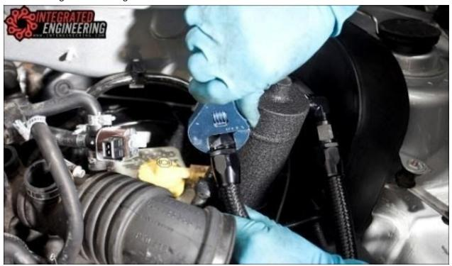
Install the supplied catch can filter.
