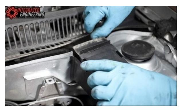
Install the corresponding relays back into their correct colored housings.
