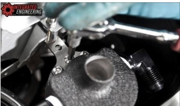
Tighten the straight AN fitting on the hose coming from the block breather to the catch can.
