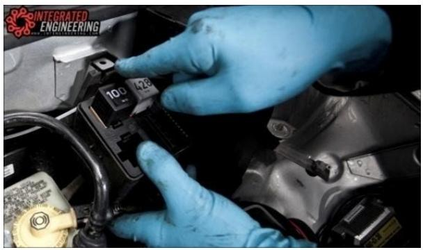
Remove the upper half of the relay box and both relays #100 and #428.
