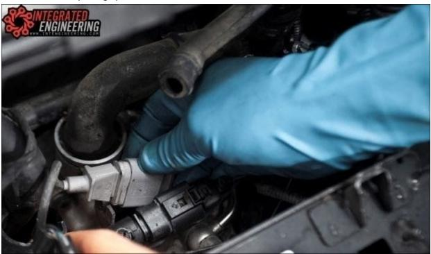
Remove the green U clip that secures the breather hose coming from the oil filter housing. *Make sure* you do not lose this clip as you will need it for reinstallation.
