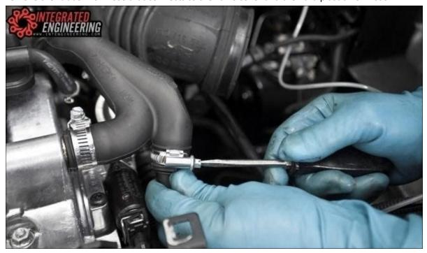
There are three ports on the suction jet pump located under the intake manifold. There are two straight barbed ends on each end of the pump and one that branches off at a 45 degree angle. Cut the clamp that secures the hose on the suction jet pump that runs in the 45 degree direction).
