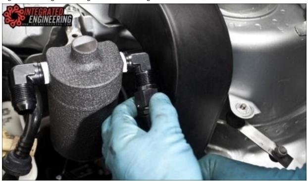
Remove the bung that is connected to the valve cover. Using a pair of pliers rotate the bung in a clockwise and counter clockwise fashion, while pulling the bung to the driver fender.
