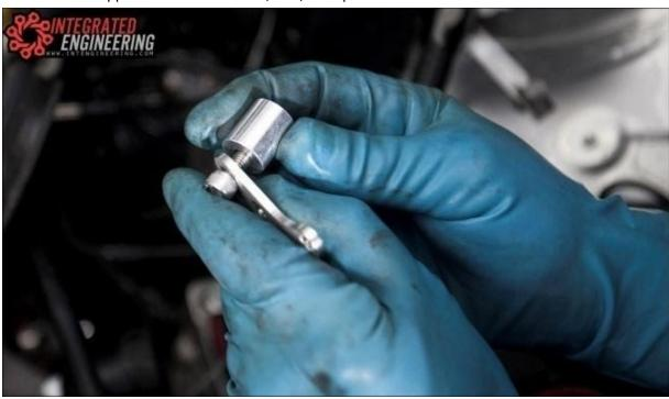
Install the bracket in the location of the relay box as seen below. You will need a 5mm allen wrench and 10mm wrench.
