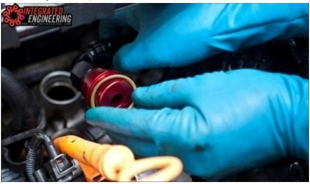
Install the adapter back into the breather housing with the catch can hose pointed to the driver side.
