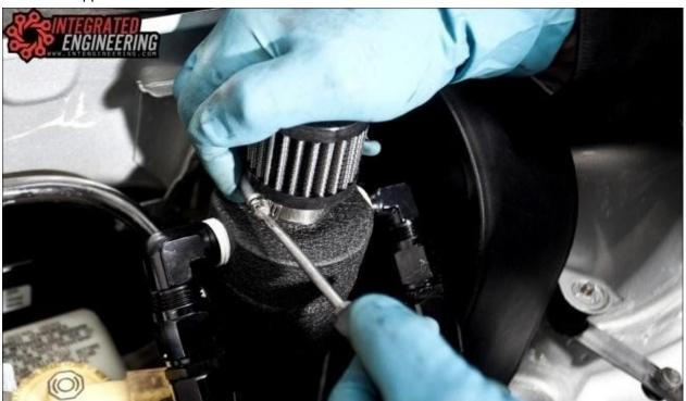
Reinstall the MAF, diverter valve, and intake. Make sure that the MAF is installed in the correct position so that drivability problems are not an issue. If everything is installed correctly the engine compartment should look as follows. Make sure that the catch can hoses do not impede the travel of the shift tower or linkages. If this is the case make minor adjustments to the hoses.
