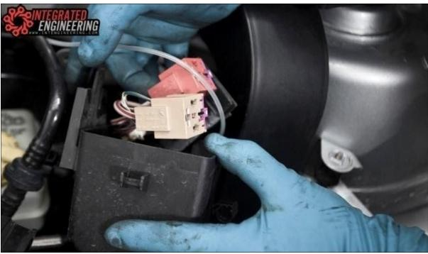
Remove the weather strip that runs along the rain tray. Remove the main wiring harness cover by releasing the mounting tabs located at the top of the cover. Use a small screwdriver and gently pry the tabs apart on both sides of the cover as shown. Lift the rain tray up and gently pull the cover out from underneath the rain tray. Remove the cover from the vehicle.
