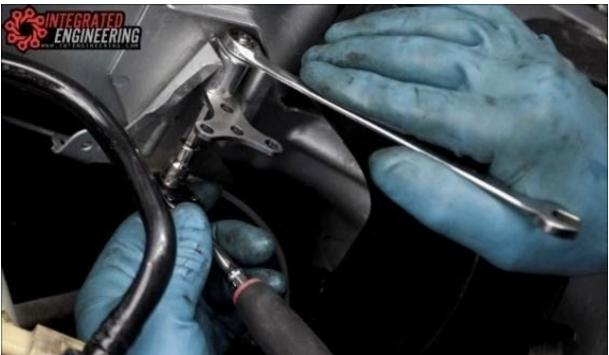
Remove both of the -10 AN to  $\frac{1}{2}$ " pipe fittings from the hose ends. Apply a light layer of Teflon tape to the hose ends and install onto the catch can until the fittings are snug. Point the fittings at a downward angle.
