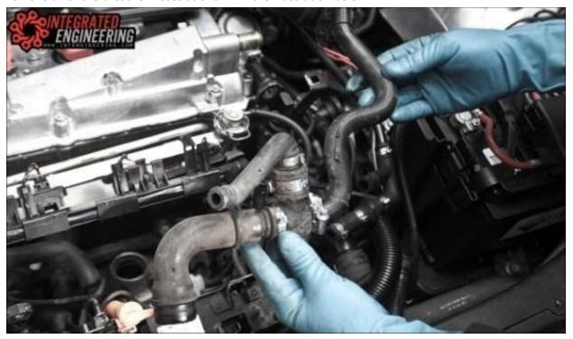
Carefully remove the o-ring located at the top of the breather housing. *Make sure you do not lose this o-ring as you will need it for reinstallation.*
