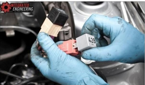
In this step, great attention and detail must be taken as to not damage any of the wiring. Carefully with a razor knife cut away the electrical tape that attaches the grommet that was removed from the relay box.
