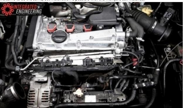
Start by removing the MAF from the turbo inlet hose. After the MAF has been removed, unclip the MAF wiring retainer located on the relay box.
