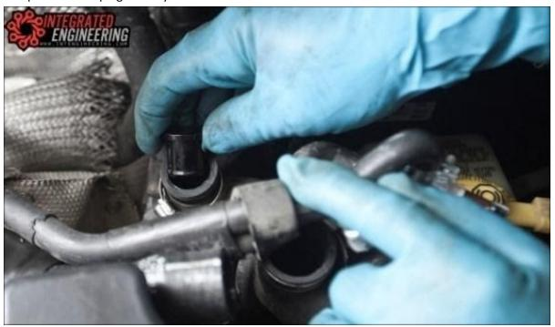
Remove the rubber PCV hose that connects to the valve cover and the hard plastic PCV hose.
