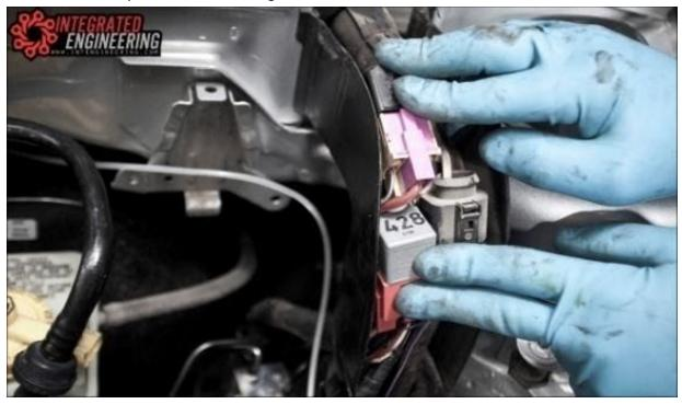
Reinstall the cover. The relays make installing the cover tight fit, but with a little finesse and patience it is possible.
