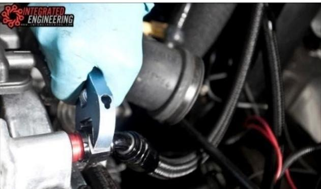
Route the breather hose under the turbo inlet hose and connect the straight AN fitting to the catch can. At this time tighten the fittings to the catch can.
