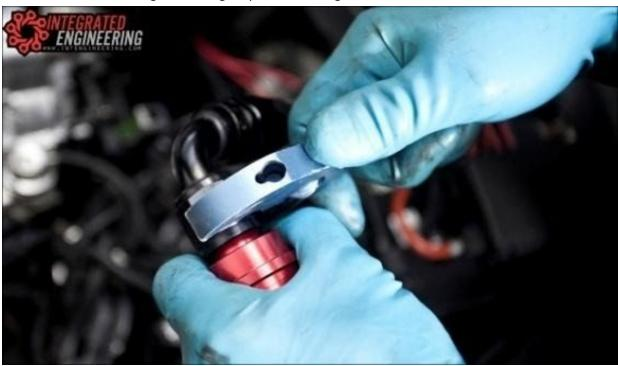
Install the o-ring onto the adapter as shown.
