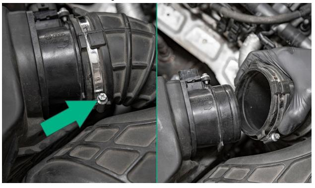
Pull to disconnect the airbox from the fender clip, then pull up to remove the entire airbox from the vehicle.
