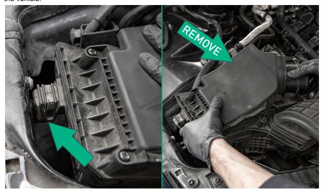
Pull to remove both factory rubber grommets from the bottom side of the airbox. Set these aside as you will reuse them later.
