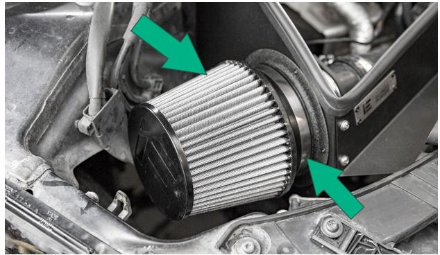
Reinstall the valve cover, verify all hose clamp connections are tight, and that your intake is fully installed. Start the car and inspect for any leaks or rubbing components. Enjoy the performance, looks, and sound of your new IE Cold Air Intake!.
