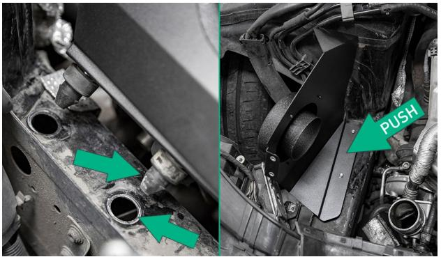
Push the front support bracket bushing into the rubber grommet on the front support bracket assembly. *This may already be done, if so, skip this step.*
