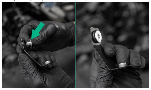
Using a T30 Torx driver and included screw, install the front support bracket to the radiator support as seen below.
