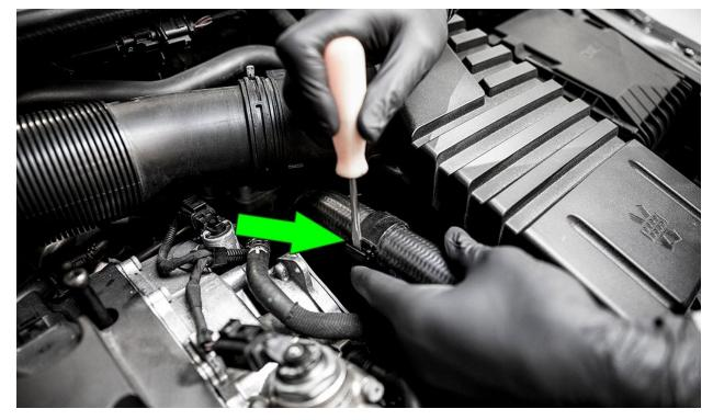
Use a pair of pliers, or hose clamp pliers, to remove the hose clamps located on the MAF housing and turbo inlet pipe. Remove the hose.
