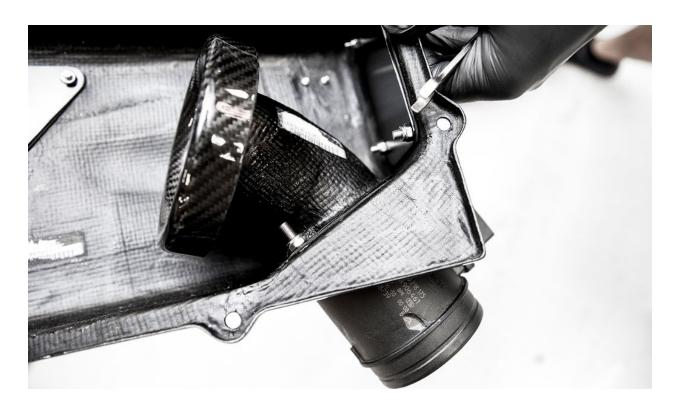
Now install the air filter onto the carbon fiber velocity stack using the large hose clamp. Once the filter is flush with the back of the velocity stack tighten the clamp firmly. As usual, do not over tighten.
