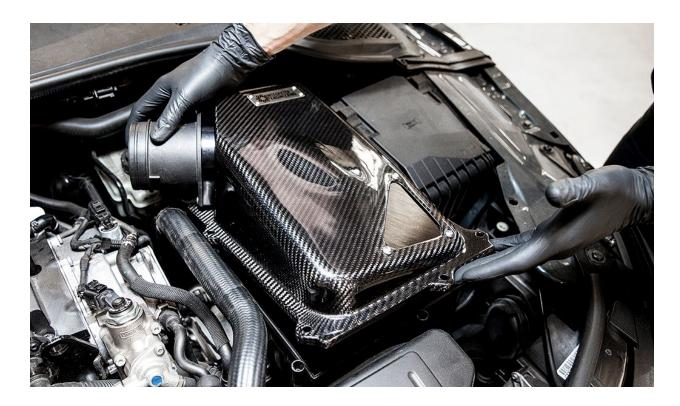
Reinstall the 8 phillips screws that were removed from the stock intake lid earlier. Tighten these bolts firmly, being careful not to over tighten causing damage the threads on the lower air box or the carbon on the IE intake lid.
