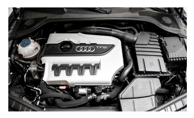
Start the installation procedure by removing the engine cover. This is done by pulling up firmly on both sides.
