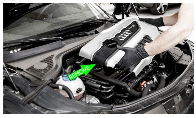
Remove two clips on the diverter valve hose by pushing on the alligator tabs with a flat head screwdriver and place the diverter valve hose off to the side. Unplug the MAF sensor by pulling back on the clip with your thumb.
