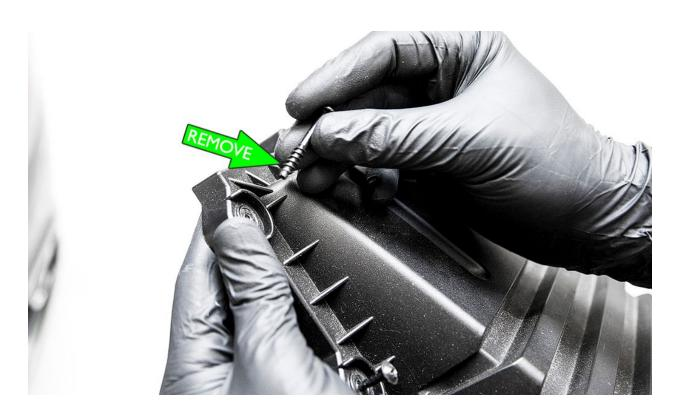
Remove the MAF housing from the stock airbox by removing the 2 phillips screws. Keep the MAF housing as you will be reusing it on your IE airbox lid.
