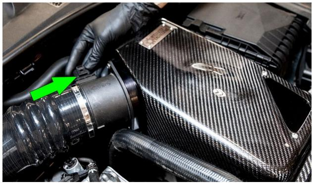
Adjust the hump hose to fit correctly between the factory inlet pipe and MAF housing and tighten the hose clamps on both ends.
