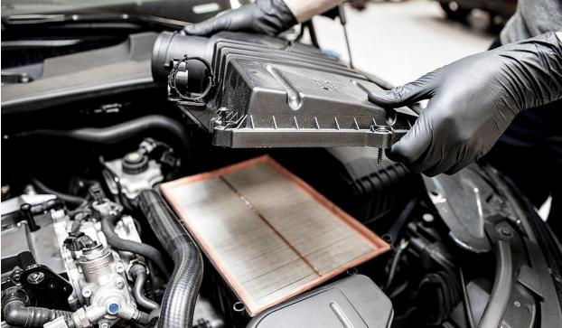
With the stock airbox lid off the car, fully remove the 8 phillips screws. Keep these as they will be reused on your new IE airbox lid.
