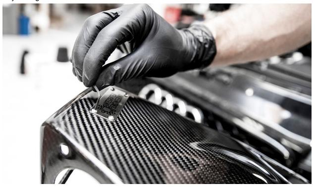
OPTIONAL STEP - If you want to install the sound doors for a quieter driving experience, use the supplied gaskets, black noise doors, M6X14mm button head cap screws, and M6 nylon insert locknuts. The sound doors and gaskets go on the inside of the airbox with the gasket against the carbon fiber. Tighten the bolts and nuts using a 4mm allen wrench and 10mm socket or wrench. Again, do not over tighten to avoid damaging the carbon fiber
