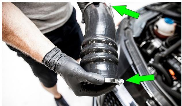
Now install the hump hose that connects the MAF housing to the turbo inlet pipe and clip the MAF connector back into the MAF housing.
