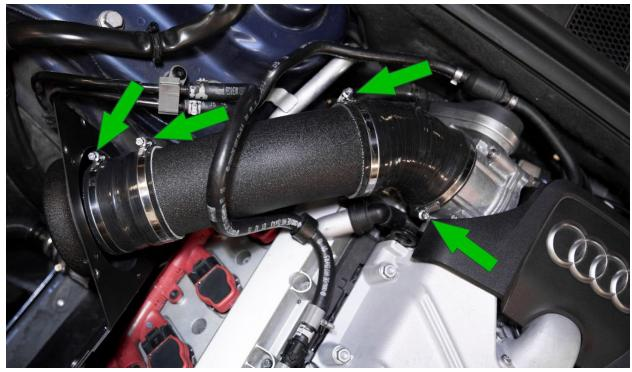
Push to install the factory vacuum line to the new IE inlet silicone. Secure with a zip tie.
