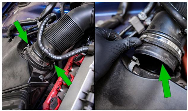
Pull back on the airbox to disconnect it from the fender bracket, then pull up to disconnect the box from the lower grommets. *Do not completely remove the airbox in this step.* **Optional Step:** You may remove the side fender bracket with a T30 torx driver for a cleaner look.
