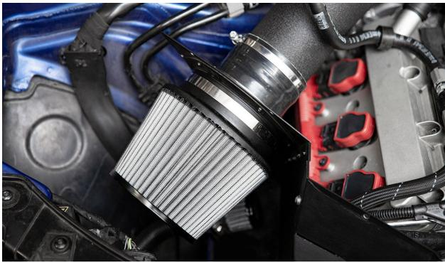
Re-install the air snorkel using a T25 torx driver and factory bolts.
