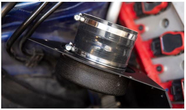
Line up the heat shield and grommets with the install location on the frame rail. Push down on the heat shield and lock in the grommets.
