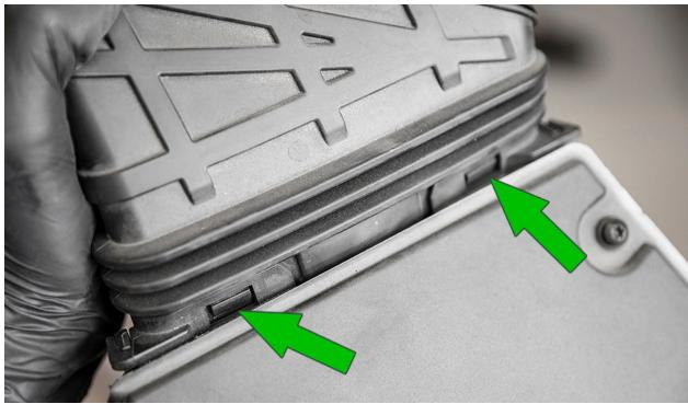
The snorkel joint connecting it to the airbox now needs to be removed. Depress the clips on both sides of the snorkel then separate the halves.
