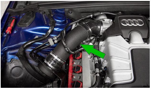
Once you are happy with the intake position, firmly tighten all hose clamps with a screwdriver. Do not over-tighten hose clamps.
