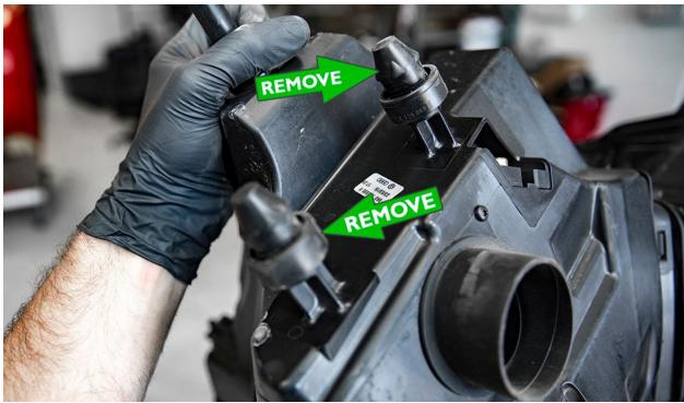
You will need to remove the factory snorkel from the stock airbox for reinstall, begin by disconnecting the clips on both sides of the snorkel.
