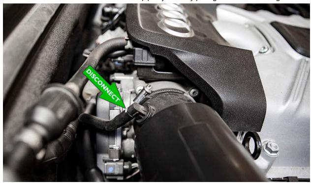
Using a flat head screwdriver, loosen the hose clamp and remove the stock intake pipe from the vehicle.
