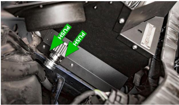
Align the heat shield with the installed IE support bracket, and install using the included M6 allen head bolt and washer with a 4mm allen wrench.
