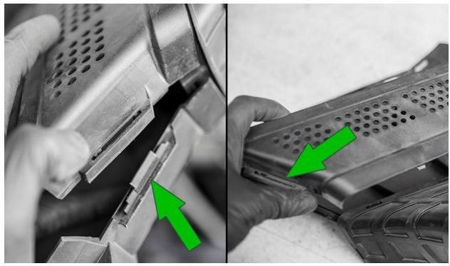
With the halves separated, remove the snorkel joint.
