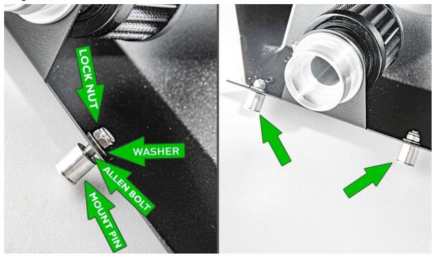
Install the factory grommets onto the IE mount pins.
