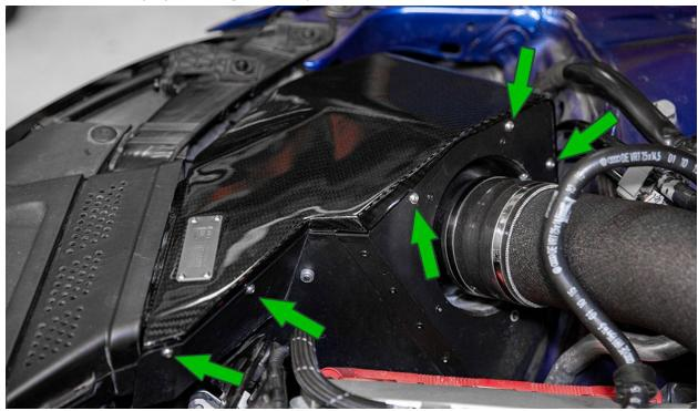
Re-install the radiator cowel and push clips. Verify all hose clamp connections are tight, and that your intake is fully installed. Start the car and inspect for any leaks or rubbing components.
