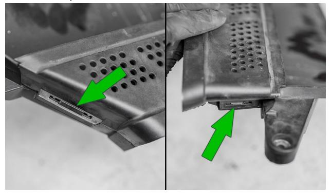
Pull up on the hose clip to release the fuel line from the intake pipe, safely set fuel line outside the clip.
