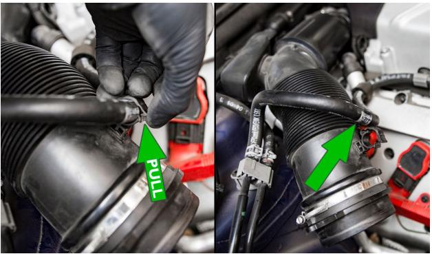
Carefully pull to release the EVAP line from the rear of the intake pipe.
