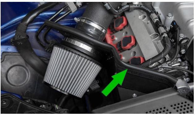
To install CF lid, line-up the lid with the heatshield mount holes. By hand, thread in the supplied button head bolts and washers starting from the outside edges and working in. Once all bolts are threaded loosely by hand, tighten firmly with a 2.5mm allen. *Do not overtighten bolts!*
