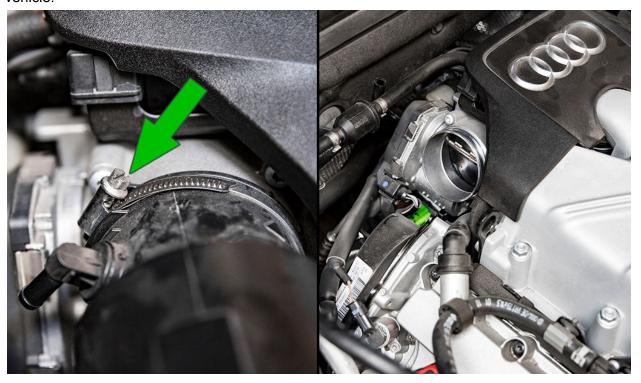
Insert the SAI adapter into the SAI bracket on the heatshield. Install the SAI filter and clamp onto the adapter, sandwiching the bracket then tighten the clamp with a screwdriver. The filter should be sitting facing the heat shield when installed.
