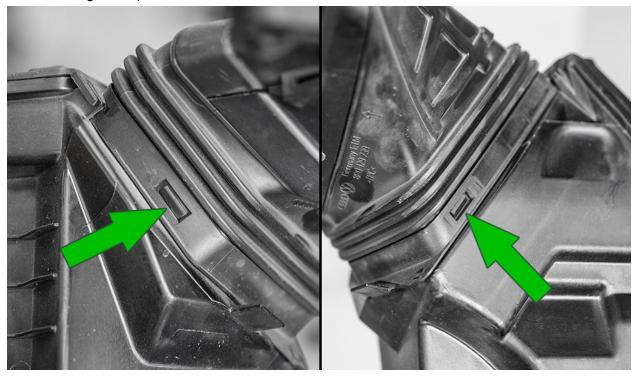
Depress the two clips on the top-side of the snorkel, this will completely disconnect the snorkel assembly from the airbox..
