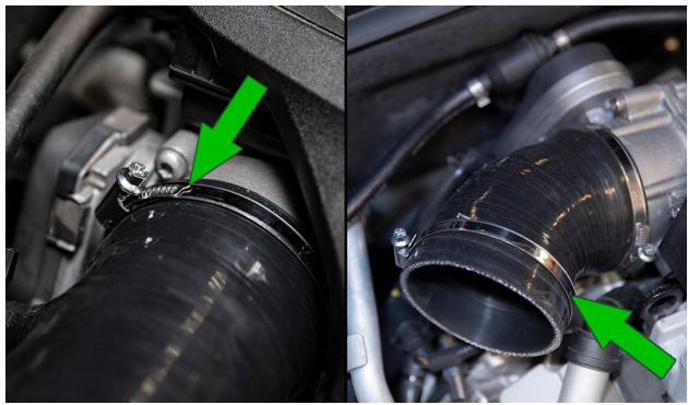
Loosely install the 80-100mm clamps and velocity stack silicone to the velocity stack on the heatshield. *Do not tighten hose clamps in this step*.
