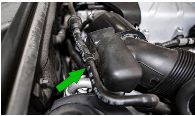
Disconnect the vacuum line from the intake pipe by carefully pulling it off the barb fitting.
