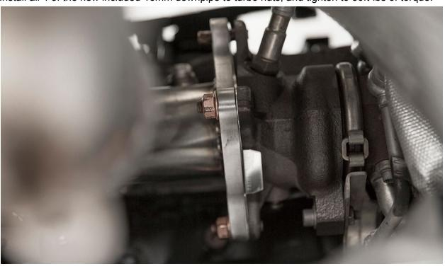
Re-install the downpipe mount bracket with the 2 factory 13mm bolts.
