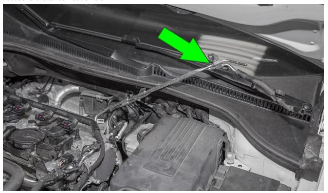
Using a socket wrench and 6mm hex driver, loosen the 3 bolts securing the heat shield to the cylinder head. Once loose, remove heat shield.
