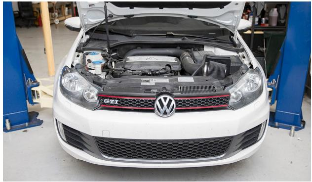
Begin the install by removing the factory engine cover and installed cold air intake system to gain access to the rear turbo heatshield.
