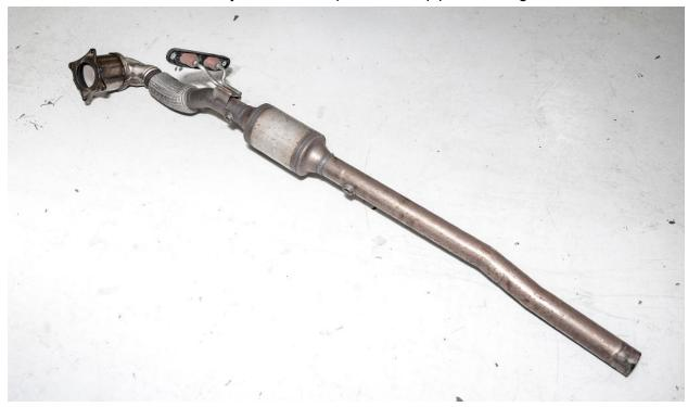
Using a small flathead screwdriver or automotive pick, carefully pry the downpipe mount bracket off the factory downpipe.
