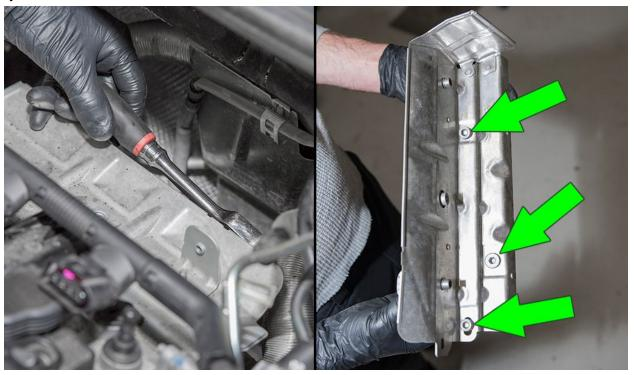
Remove the two upper 16mm nuts from the downpipe to turbo flange.
