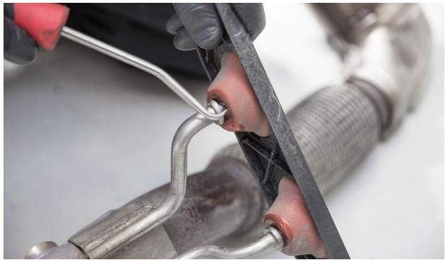
Line-up the included IE downpipe bracket, and press it fully into the factory mount grommets.
