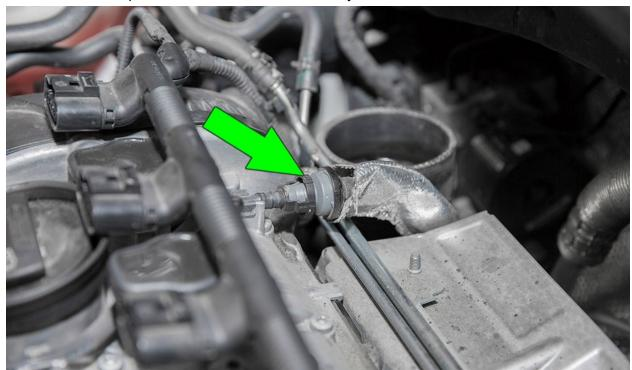
Remove the T30 torx bolt from the coolant crossover pipe. This bolt is located on the back of the cylinder head just above the turbocharger. A mechanic's mirror may help if you have a hard time locating it.
