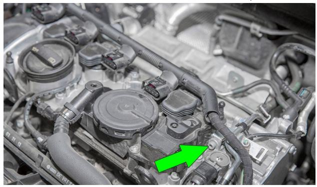
Loosen the coolant bottle cap to release pressure from the system. Using pliers or spring clamp removal tool, disconnect the coolant over flow line from the coolant bottle.
