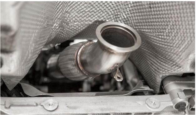
Install all 4 of the new included 16mm downpipe to turbo nuts, and tighten to 30ft-lbs of torque.
