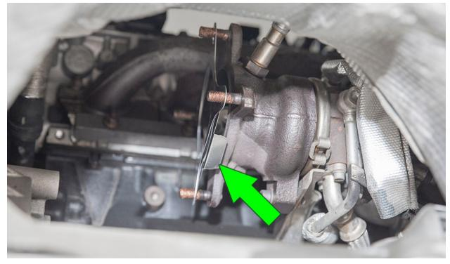
If your top 02 sensor is located in the turbo, install the supplied 02 plug. If your 02 sensor is located in the downpipe, skip this step.
