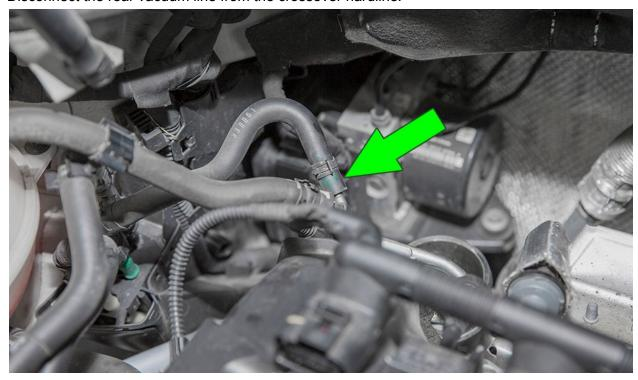
The crossover hardline should now be loose, carefully place it out of the way so you gain full access to the turbo heat shield.
