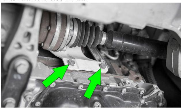
Re-install chassis braces with factory 13mm nuts.
