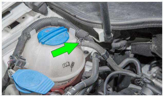
Disconnect the rear vacuum line from the crossover hardline.
