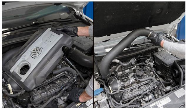
Remove the #8 triple square bolt from the top of the heatshield.
