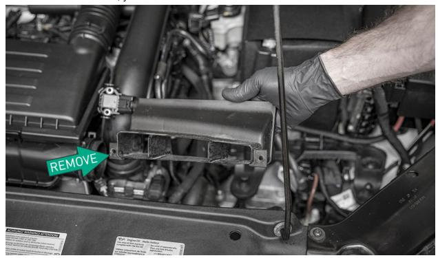
Carefully pull back on the vacuum line to disconnect it from the air box.
