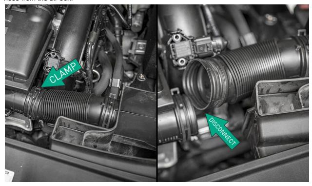
Disconnect both tabs on the air snorkel with a flathead screwdriver to release it from the front inlet.
