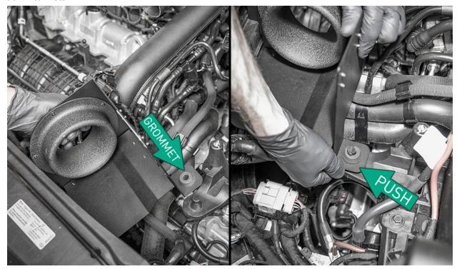
Install the larger rubber insert grommet and aluminum sleeve to the heatshield bracket with the larger side facing the front of the vehicle. Install to the radiator support with included T25 screw and large washer.
