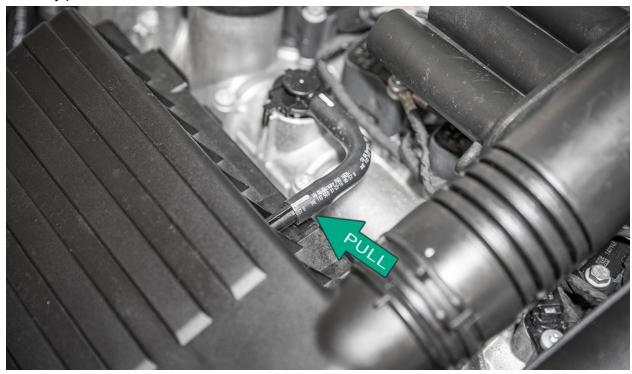
Release the hose clamp and disconnect the airbox to turbo inlet pipe.
