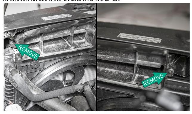
With the screws removed, you can now remove the air inlet from the front of the vehicle.
