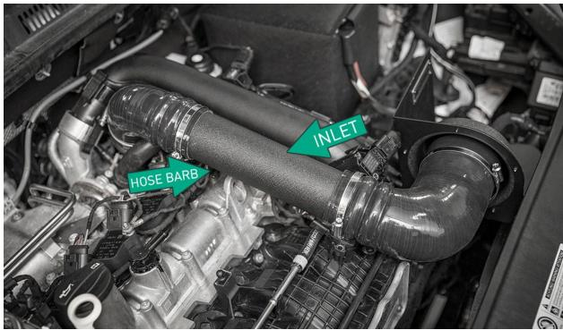
Adjust the position of the intake silicone and inlet making sure it is not pulling or bound and that it sits freely and without tension. Once you are happy with the intake position, firmly tighten all hose clamps with a screwdriver. *Note: Do not over-tighten hose clamps*.
