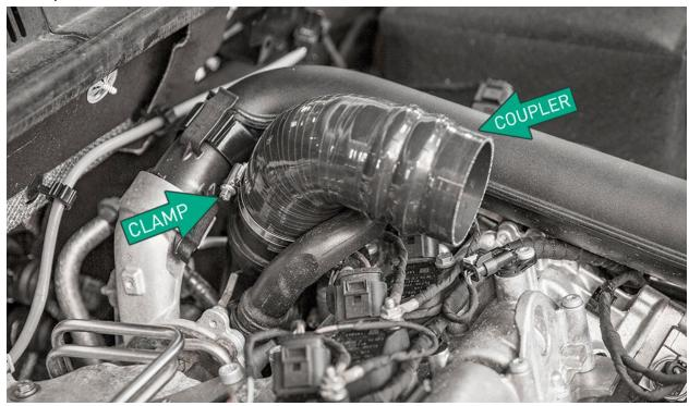
Install the 90 degree velocity stack coupler to the IE heatshield with 80-100mm clamp. *Note: Do not tighten hose clamps in this step.*
