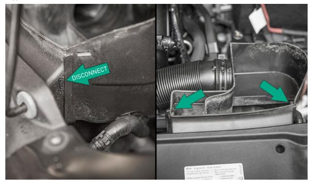
When the two halves are separated, remove the air snorkel from the vehicle.
