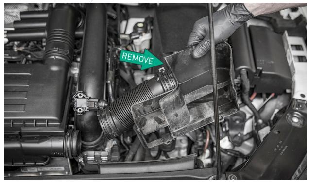
Remove both T25 screws from the sides of the front air inlet.
