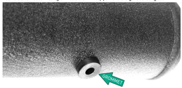
Install the IE inlet pipe and both 50-70mm hose clamps. Install the 90 degree hose barb to the rubber grommet insert closest to the turbo side.
