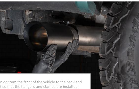
Install the tip, then go from the front of the vehicle to the back and adjust the exhaust so that the hangers and clamps are installed properly. Once everything is oriented correctly, tighten all the clamps to 42 ft/lbs. Installation is now complete! Enjoy the look, sound, and performance of your new Xodus Catback Exhaust!
