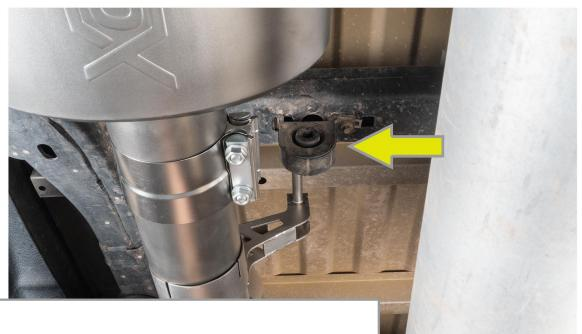
Ensure the hanger is installed on the middle hanger isolator. Lubrication may help.
