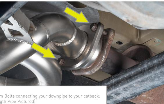
Remove two 16mm Bolts connecting your downpipe to your catback. (Xodus Equal Length Pipe Pictured)
