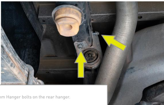
Remove two 13mm Hanger bolts on the rear hanger.
