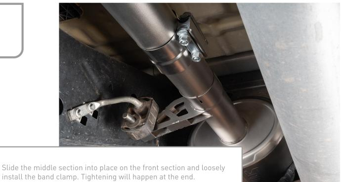
install the band clamp. Tightening will happen at the end.
