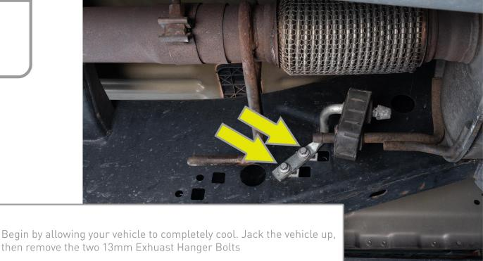
then remove the two 13mm Exhuast Hanger Bolts
