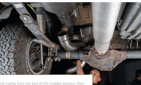
Slide provided band clamp onto the exit of the middle section, then lift the rear section into place over the axle and slide it into place on the middle section.
