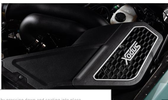
Install intake lid by pressing down and seating into place.
