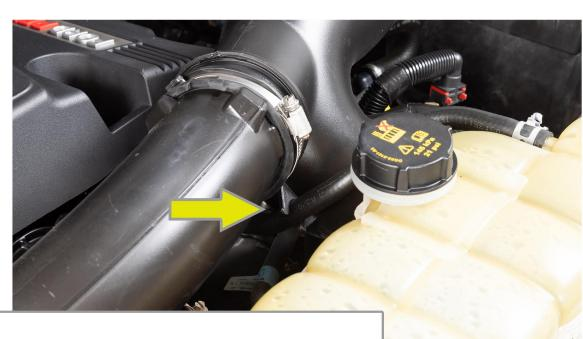
Release coolant hose from lower turbo inlet pipe.
