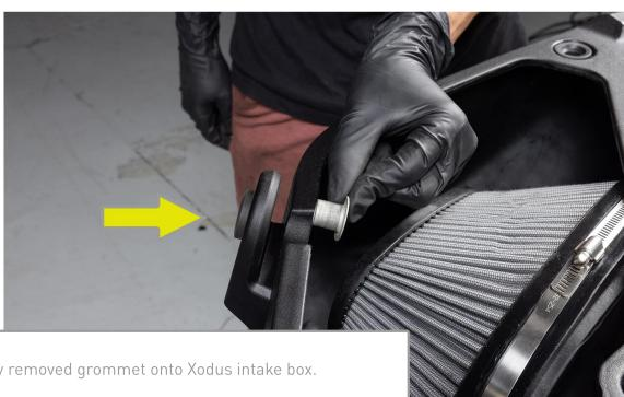
Install previously removed grommet onto Xodus intake box.
