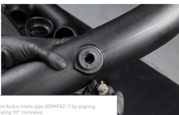
Install sensor onto Xodus intake pipe (XOINFA2-1) by aligning channels and rotating 90° clockwise.
