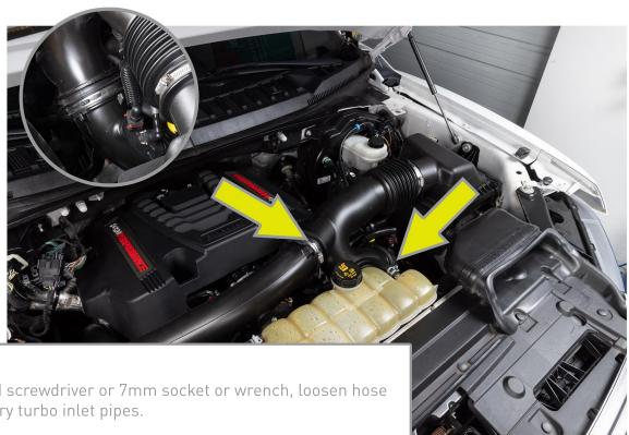
Using a flathead screwdriver or 7mm socket or wrench, loosen hose clamps on factory turbo inlet pipes.
