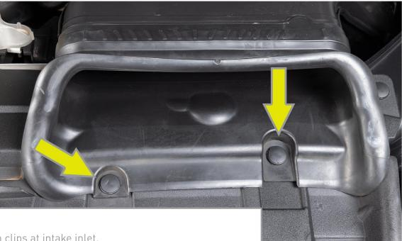
Remove two push clips at intake inlet.
