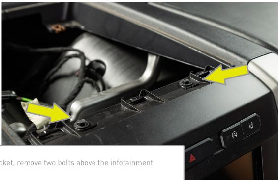
Using a 7mm socket, remove two bolts above the infotainment screen.
