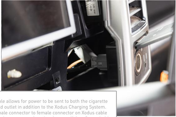
The included cable allows for power to be sent to both the cigarette lighter/household outlet in addition to the Xodus Charging System. Plug in factory male connector to female connector on Xodus cable and plug male Xodus connector into the cigarette lighter/household outlet connector behind air vent.
