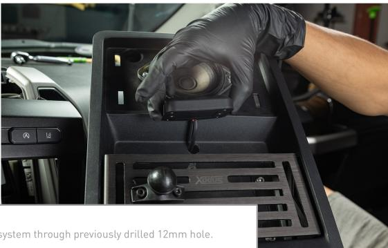
Insert Charging system through previously drilled 12mm hole.
