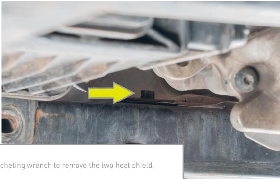
Use a 10 mm ratcheting wrench to remove the two heat shield, retaining bolts
