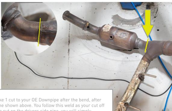
You will now make 1 cut to your OE Downpipe after the bend, after the Cat on the line shown above. You follow this weld as your cut off point. There is no cut on the drivers side pipe, you will simply remove a band clamp.
