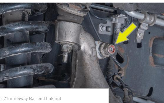
Remove the upper 21mm Sway Bar end link nut
