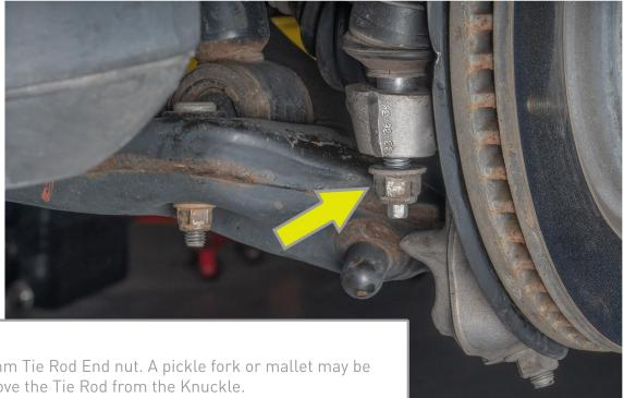
Remove the 21mm Tie Rod End nut. A pickle fork or mallet may be required to remove the Tie Rod from the Knuckle.
