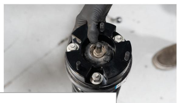
Install your Xodus Leveling Kit on top of the strut and fasten it to the strut using the OE Nuts
