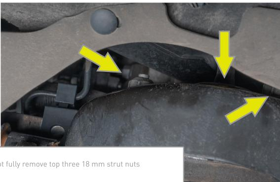
Loosen but do not fully remove top three 18 mm strut nuts
