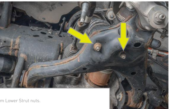
Remove two 18mm Lower Strut nuts.
