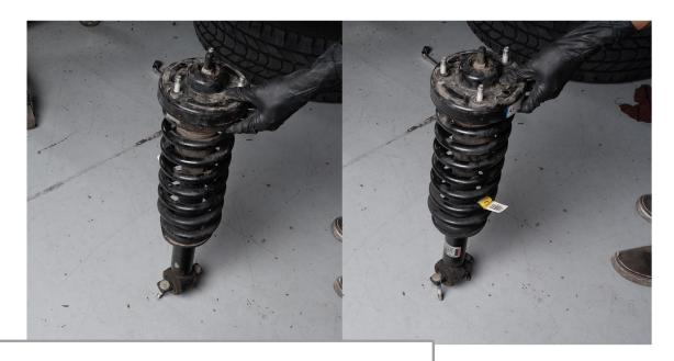
Once the strut is out, if you have **NON ADAPTIVE** suspension, simply rotate the strut 180° From it's Original orientation.
