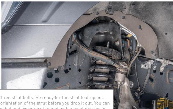
Remove the top three strut bolts. Be ready for the strut to drop out. Take note of the orientation of the strut before you drop it out. You can even mark the top hat and lower strut mount with a paint marker to know which side was facing outward. Note that you may need to apply upward pressure on the knuckle to allow clearance for the strut.
