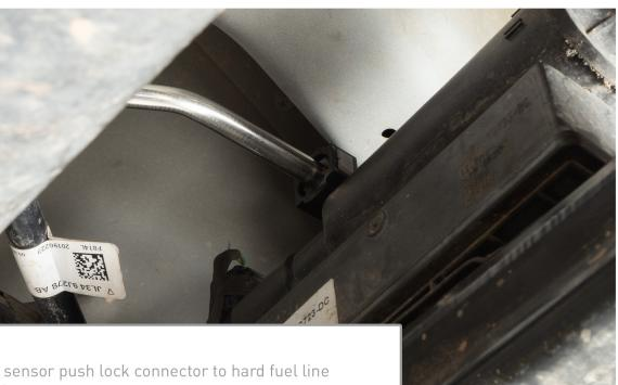
Connect Trueflex sensor push lock connector to hard fuel line underneath vehicle.
