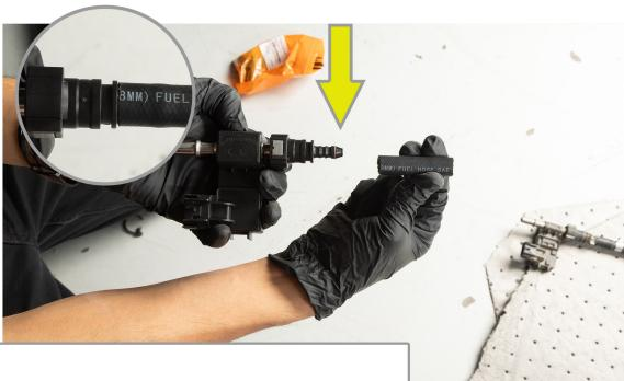
Press included fuel hose onto previously installed push lock connector barb. Be careful to make sure brown o ring does not unseat from barb. Push hose until it is flush with the end of the barb.
