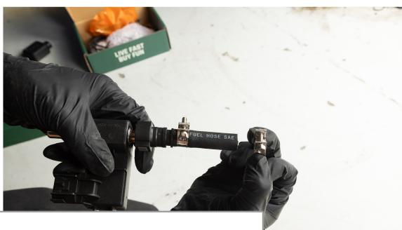
Install two included clamps onto fuel hose. Tighten inner clamp using a 7mm or flat head screwdriver.
