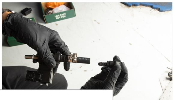
Install second push lock connector onto fuel hose, be careful not to unseat brown o ring on barb. Tighten second clamp with a 7mm or flathead screwdriver.
