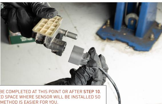
THIS STEP CAN BE COMPLETED AT THIS POINT OR AFTER STEP 10. THERE IS LIMITED SPACE WHERE SENSOR WILL BE INSTALLED SO USE WHATEVER METHOD IS EASIER FOR YOU.
