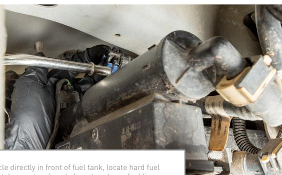
Underneath vehicle directly in front of fuel tank, locate hard fuel line. Spread blue tabs apart and push down to release fuel line. There may be residual fuel in lines, so be prepared and wear safety glasses.
