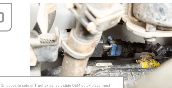
On opposite side of Trueflex sensor, slide OEM quick disconnect onto sensor quick disconnect. This connector will not click into place. Slide blue tab back down to lock into place. Confirm connector is locked into place before moving forward.
