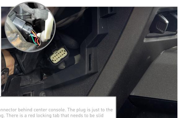
Unplug 12 pin connector behind center console. The plug is just to the left of the opening. There is a red locking tab that needs to be slid open in order to unplug.
