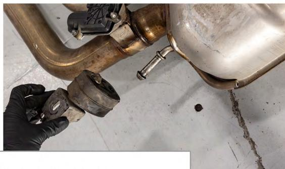
Remove both exhaust hangers from stock exhaust.
