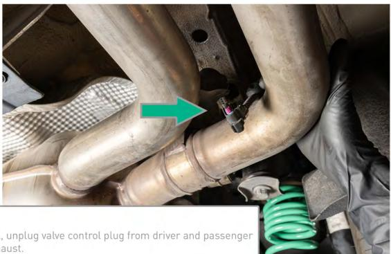
Using a pick tool, unplug valve control plug from driver and passenger side of stock exhaust.
