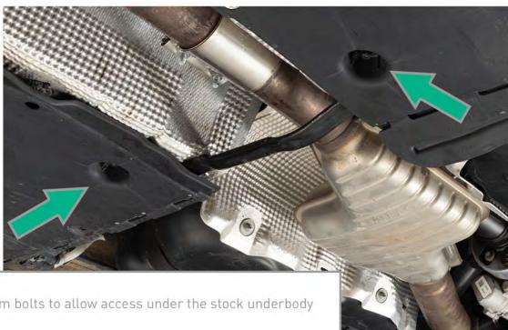
Remove 2 - 10mm bolts to allow access under the stock underbody tray.
