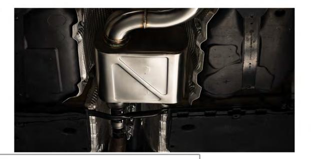
Reinstall cross brace using 4 - 13mm nuts. Secure underbody tray using 10mm socket.
