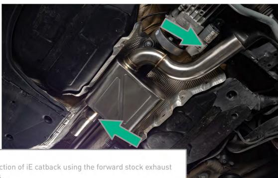
Hang muffler section of iE catback using the forward stock exhaust hanger locations.
