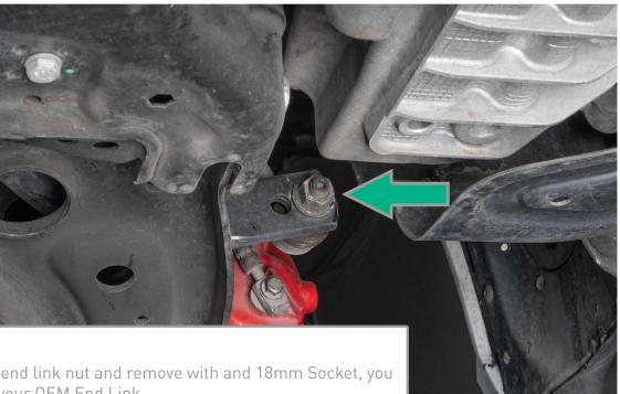
Locate the lower end link nut and remove with and 18mm Socket, you can now remove your OEM End Link.
