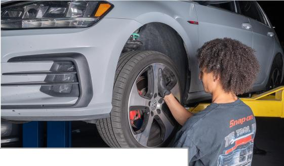
Allow your vehicle and brakes to cool, then jack up and remove the two front wheels using a 17mm socket.
