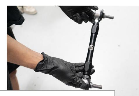
Unbox your iE Links and remove the nut from the ball joints shafts.
